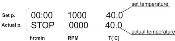
Fig.4 Control panel in operation mode
