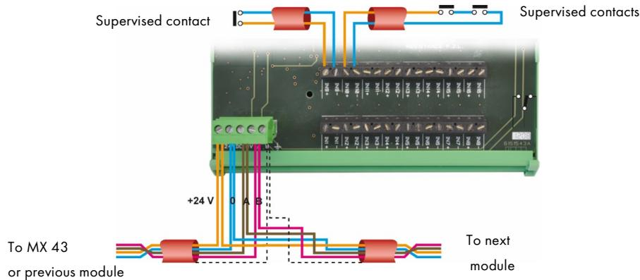
Figure 39: 16-logic input module connections.
