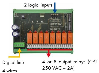
Figure 19: 8-relay module.
