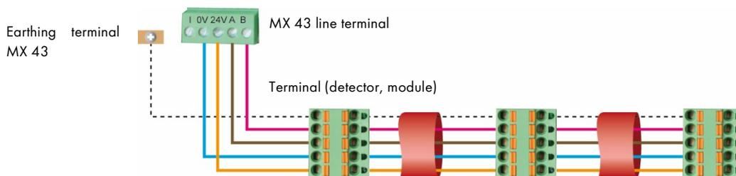
Figure 16: Principle of connecting modules to a MX 43 line.
