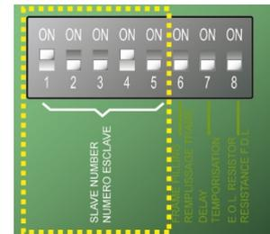
Figure 17: Switches of address configuration.
