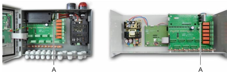
Figure 29: Connection of 24VDC external power supply (A).
