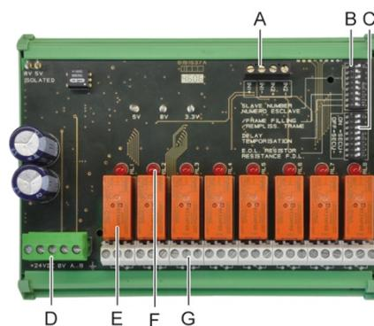
Figure 20: 8-relay module.
