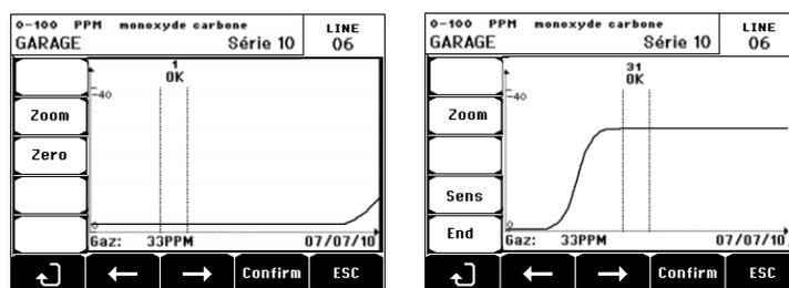
Figure 48: Adjustment of zero (left) and sensitivity (right).
