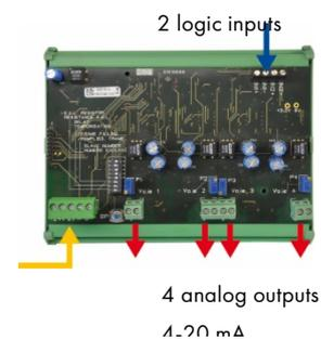
Figure 25: Principle 4-analog output module.
