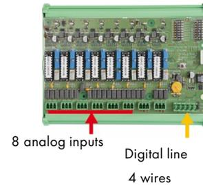
**Figure 23: 8-analog inputs.**
