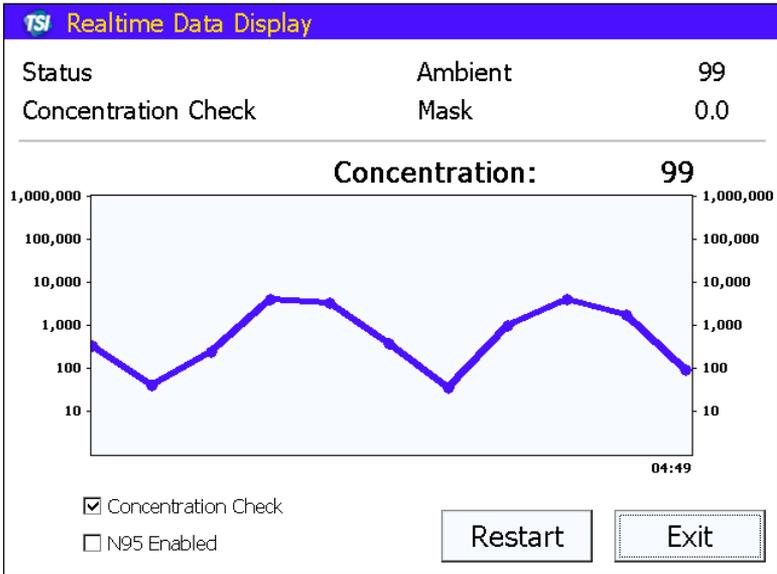
In this mode, the PortaCount Pro fit tester continuously measures the particle concentration through the ambient inlet port allowing the user to easily check ambient concentration in preparation for testing.
