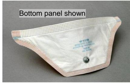
**For respirators with center-mounted exhalation valves**, install the probe to the left or right of the valve. Do **not** install the probe above or below the valve because this risks having the probe blocked by the person’s nose or chin.
