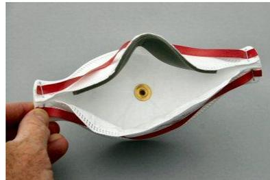
**For flat “duckbill” style respirators**, install the probe near the outer edge of the **bottom panel** where it cannot be blocked by the person’s chin.
