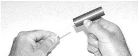
3. Examine the white Alcohol Wick. Discard wicks that are severely discolored or physically damaged. Some light brownish-yellow discoloration of the wick is normal.
