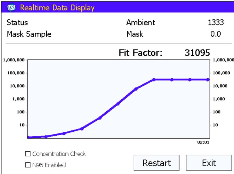
The PortaCount Pro Respirator Fit Tester takes an ambient concentration reading and stores the value. Next it purges the mask and then begins continuous monitoring of the mask concentration.
