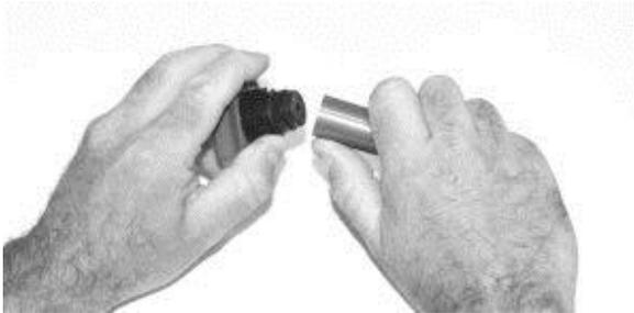
2. After separating the two halves, push the Alcohol Wick out of the Wick Retainer Cap from the opposite end with the Wick Removal Tool (wood dowel) provided with each new alcohol wick. Do **not** use a pencil point because bits of lead could break off.
