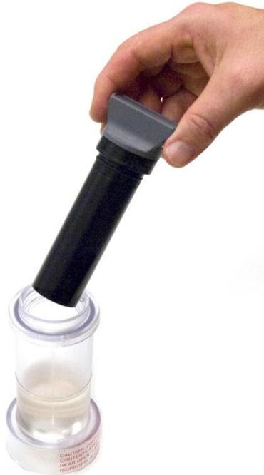
9. Set the Alcohol Fill Capsule down and wait at least 2 minutes while the alcohol wick inside the Alcohol Cartridge soaks up alcohol.
