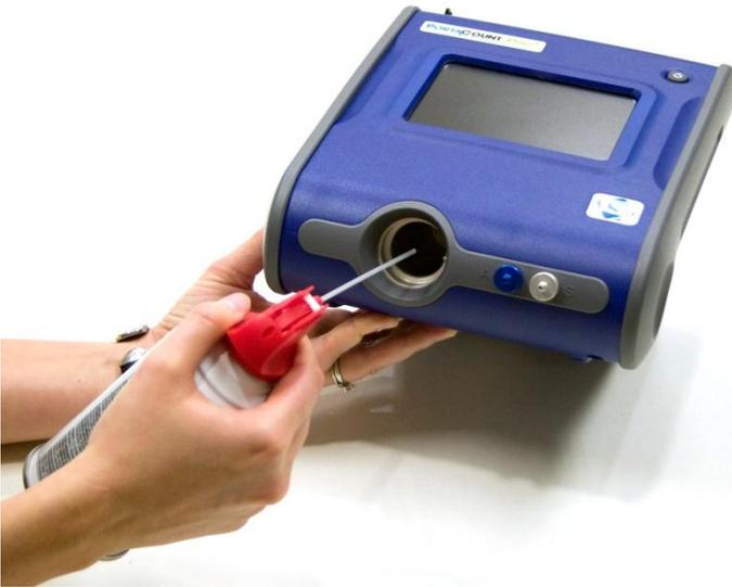
Reinsert the alcohol cartridge. Turn the PortaCount Pro Respirator Fit Tester on. Perform the Daily Checks. If the problem persists, try Procedure B.
