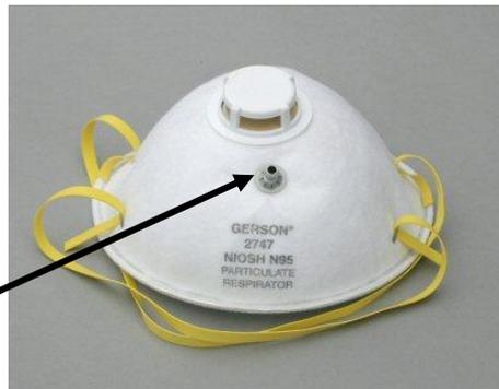
**For respirators with an outer mesh**, install the probe normally as if the mesh was not present. The sampling probe and push nut will seal properly right through the mesh.
