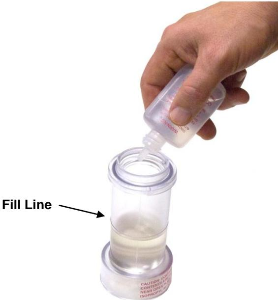
6. Squeeze alcohol into the Alcohol Fill Capsule until it is even with or slightly above the fill-line.
