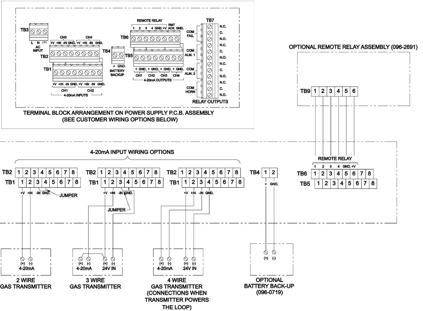
**Figure 7 – Transmitter Wiring to Model 7400**
