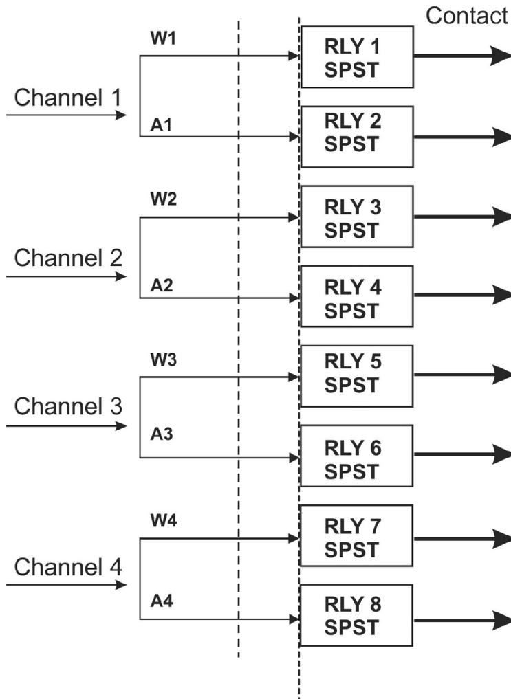
**Figure 14 - Remote Relay Settings Factory Default**
