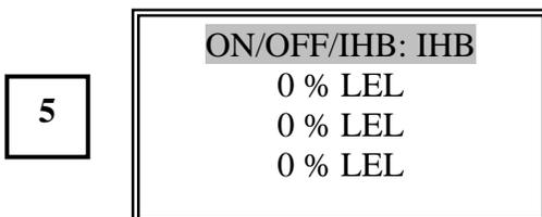
The analog output (4-20mA) will be set to the programming inhibit level. No relay contacts will activate from Channel 1. (Channel 1 was used in this example.)
