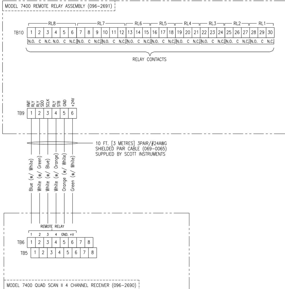
**Figure 13 - Interconnect Wiring Between 7400 & Remote Relay Assembly**
