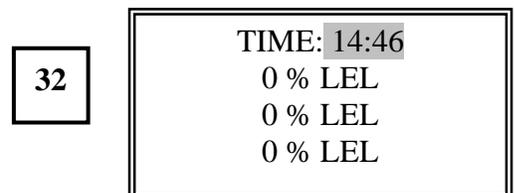
Press the **UP** or **DOWN** buttons to select the correct time. Press the **ENTER** button.
