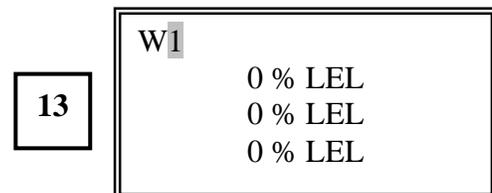
If you wish to change the 1 to another channel number, press the **UP** or **DOWN** button. If you wish to add additional alarms or **AND** and **OR** functions, press the **UP** or **Down** buttons and the **SETUP** button to move to the next position to the right on the CD display.
