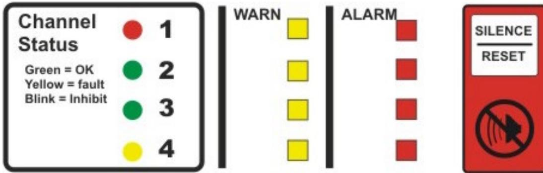
The individual visual display of absolute value of the gas concentrations, alarm status, and channel status for all active channels provides the status of the gas/flame detection system.
