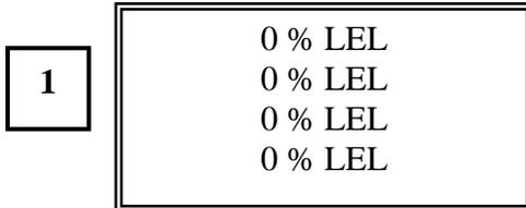
Press the **SETUP** button. This display is shown for 2 seconds.
