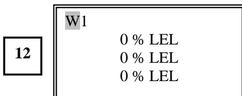
**Note 1:** To program any relay for specific alarms, the following letters, numbers and symbols are used: **W** (Warn), **A** (Alarm), **F** (Fail), **1,2,3,4**(Channel numbers), **&** (AND), **|** (OR), **(** and **)** (used to separate groups of alarms).
