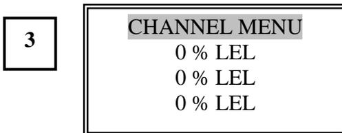
**NOTE:** From any programming point or function within the **SECURITY MENU**, **SYSTEM MENU** or **CHANNEL MENU**, you can revert back to the **Active Channel Display** by pressing **ESCAPE**.
