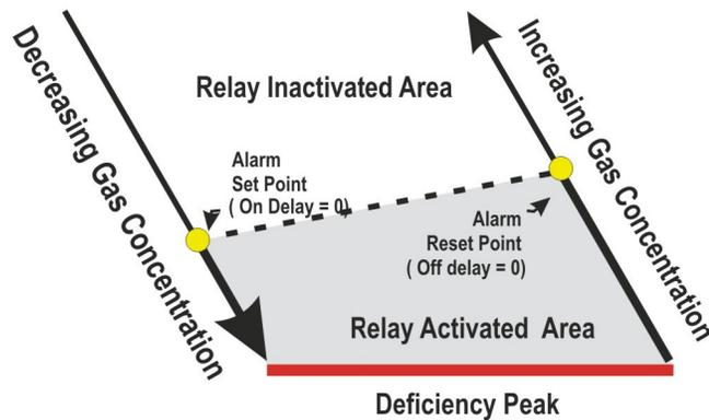
If the channel is not inhibited (channel status LED flashing), the associated relay(s) will be affected (non-energized relays will be energized, and energized relays will be de-energized). Timer activation can be set to 0 at which time relay activation will be immediate as described under Set Point.
