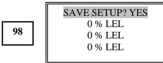
For this example select **YES**. Press the **ENTER** button. This display is shown for 2 seconds.
