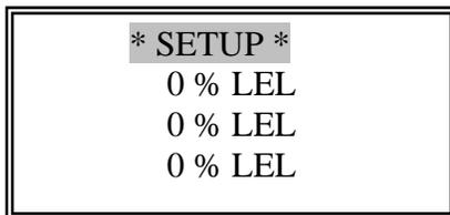
Push the **UP** or **DOWN** button to scroll through each channel. Press the **DOWN** button.
