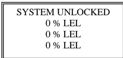
After the 2 seconds have timed out, the following Display is shown. NOTE: The shaded area on the LCD denotes a **Flashing Display** that requires **Action**.
