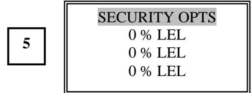
Press the **UP** or **DOWN** button to scroll through each function. Press the **DOWN** button.
