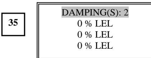
Note: The **DAMPING** may require increasing if the display is found to be unstable. Press the **UP** button
