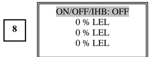
Turning a channel **OFF** drives the analog signal (4-20mA) to the programming inhibit level. No relay contacts will activate from this channel.
