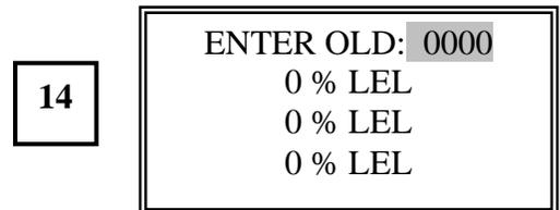
Push the **UP** or **DOWN** buttons to select your old number. Press the **DOWN** button, 9999 is displayed which is an incorrect number.
