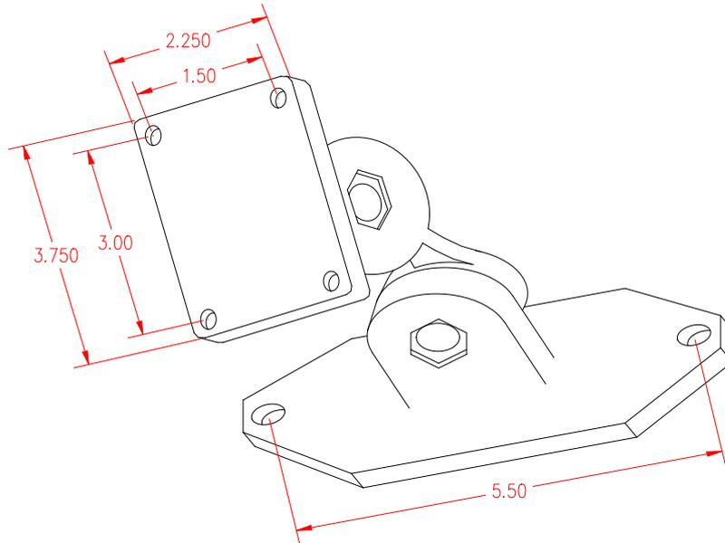
**Figure 5: Model SM4 Stainless Steel Swivel Mount**
