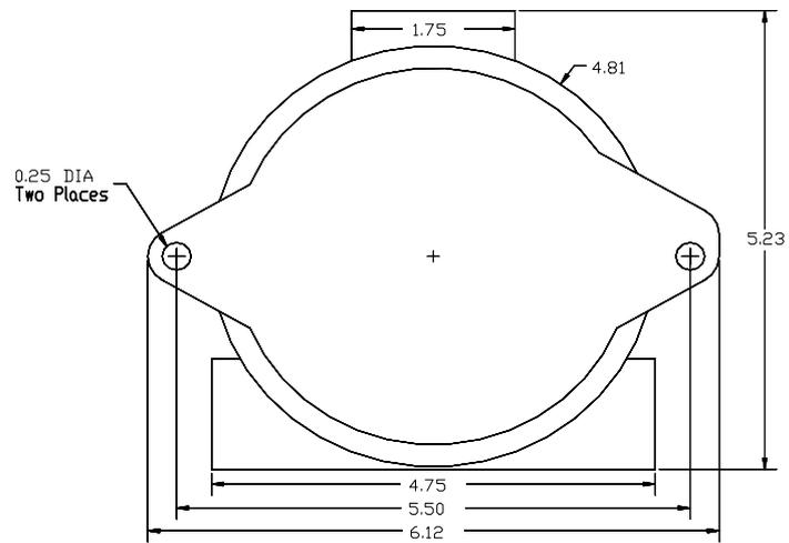
**Figure 8: Model SS4-AS/-AS2 Detector Enclosure - Rear View**
