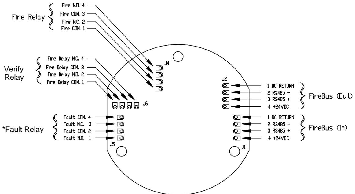
\* Fault relay is shown in the energized condition during normal operation (No Fault).
