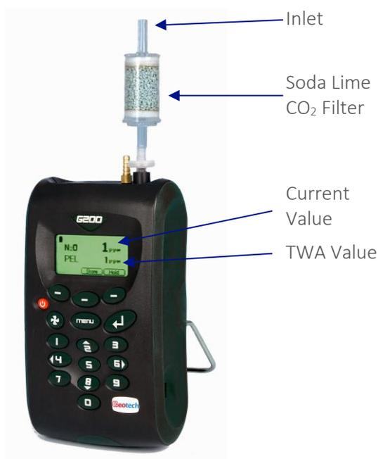
The G200 analyser is specifically designed to safety check background zone levels of N<sub>2</sub>O (0-1,000ppm) in medical applications. This instrument measures the long term exposure to N<sub>2</sub>O gas along with the TWA (time weighted average), leak detection for N<sub>2</sub>O storage. It is a dual purpose background analyser or personal analyser and is highly portable.
