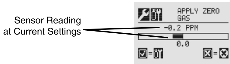
Figure 205. Apply Zero Gas screen
