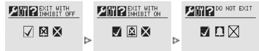
Figure 201. Span Calibration Failed
