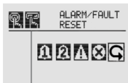
Figure 159. Alarm/Fault Reset screen
