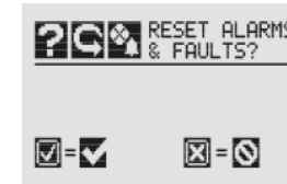
Figure 160. Alarm/Fault Reset screen
