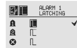
Figure 94. Alarm Latching screen
