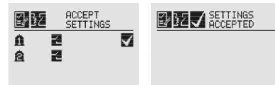
Figure 131. Accept New Alarm Relay Settings and new Settings Accepted screens
