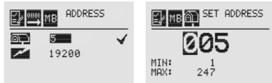
Figure 138. Set Fieldbus Address and Address Value screens
