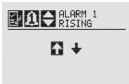
Figure 86. Setting alarm rising/falling
