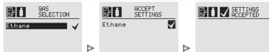
Figure 79. Select New Target Gas screens
