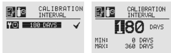
Figure 105. Edit Interval and Setting Interval Value screens
