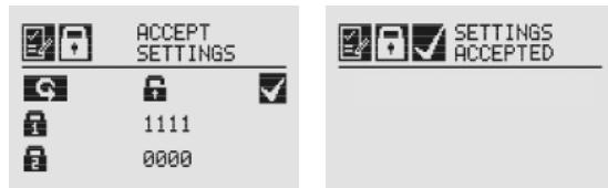
Figure 144. Accept Settings and Security Settings Accepted screens
