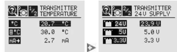
Figure 169. Transmitter Temperature and Supply Voltage screens
