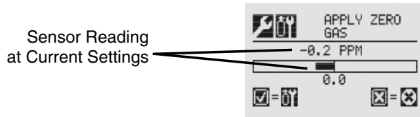
Figure 194. Zero Calibration Screen
