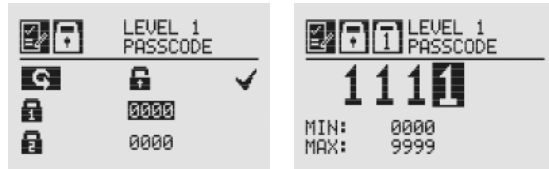
Figure 143. Setting the Level 1 passcode
