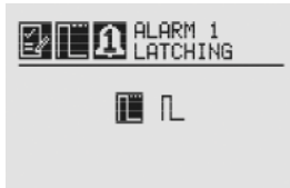
Figure 95. Setting Alarm Latching/Unlatching screen
