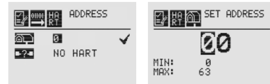
Figure 134. HART Address and Address Value screens
