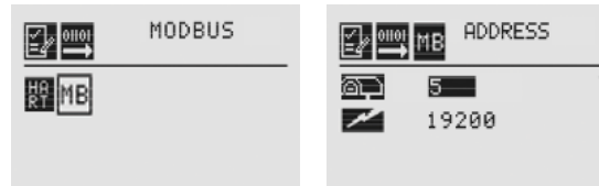
Figure 182. Modbus Configuration Display screen
