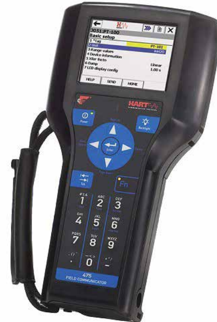
Figure 238. XNX data displayed on an Emerson field communicator
