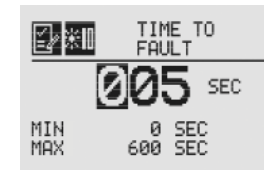
Figure 113. Setting Beam Block Fault Time screen
