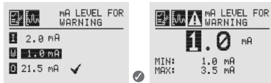
Figure 101. Set mA Levels for Warning screens
