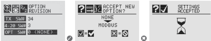
Figure 167. Updating the Transmitter for Option Boards Added or Changed screens
