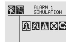
Figure 155. Alarm/Fault Simulation menu
