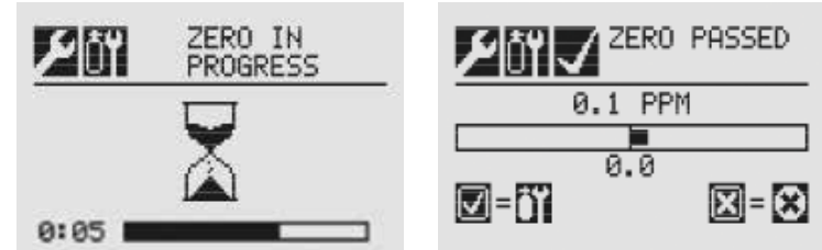
Figure 206. Zero Calibration screens
