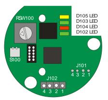
The Fire Sentry FSCHCOM-SS4 module is a piggy-back device that allows SS4-series flame detectors to communicate with a HART Network Master. The HART module may be considered to be a protocol converter. The flame detector itself communicates to external devices with the FireBus-I proprietary protocol. This HART module obtains alarm and fault status using FireBus-I, and then upon receiving a HART command will respond to the HART master by returning the necessary
