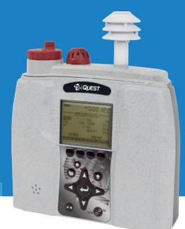
The TSI® Quest™ EVM Environmental Monitors simultaneously measure particulates and gas concentration in real-time. These monitors measure select toxic gases, volatile organic compounds (VOCs), relative humidity, temperature and air velocity.
