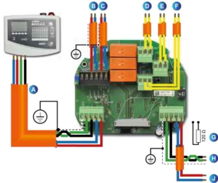
Figure 42: wiring in RS485 network topology (Modbus).
