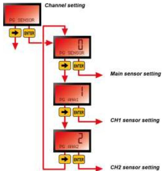
Figure 21: the *Channel Configuration* menu.
