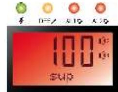
Figure 56: detection of high LEL concentration.
