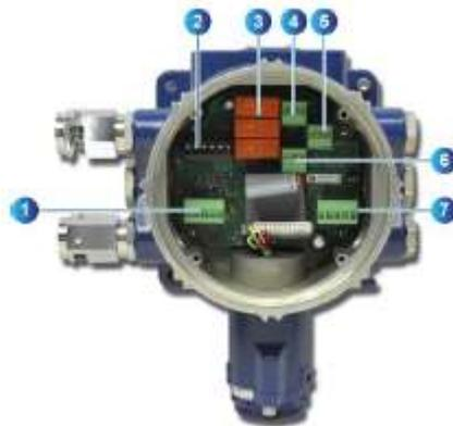
Figure 5: internal components of the transmitter.
