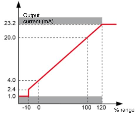
Figure 43: transfer curve for a 4-20 mA detector.
