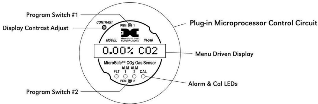
Figure 6 Control Circuit
