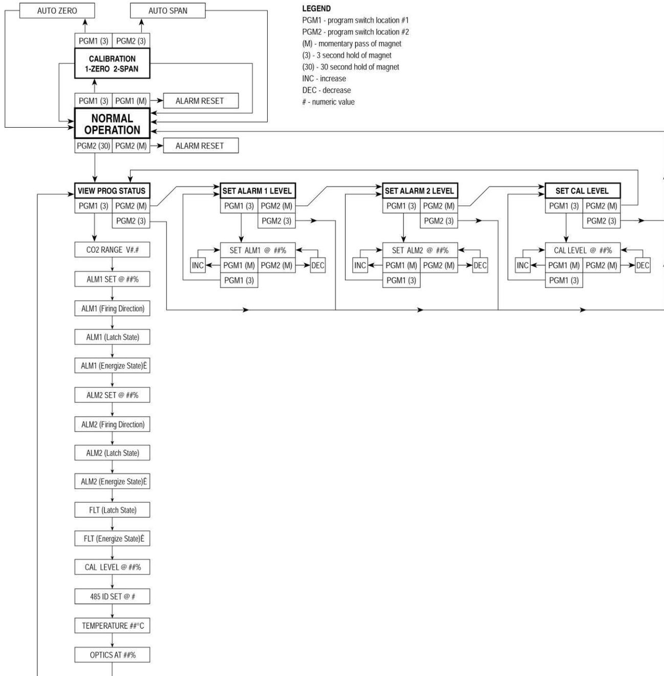
Figure 15 IR-640/IR/642 Software Flow Chart
