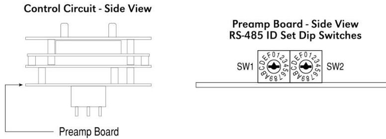
**Figure 13** RS-485 Dip Switches
