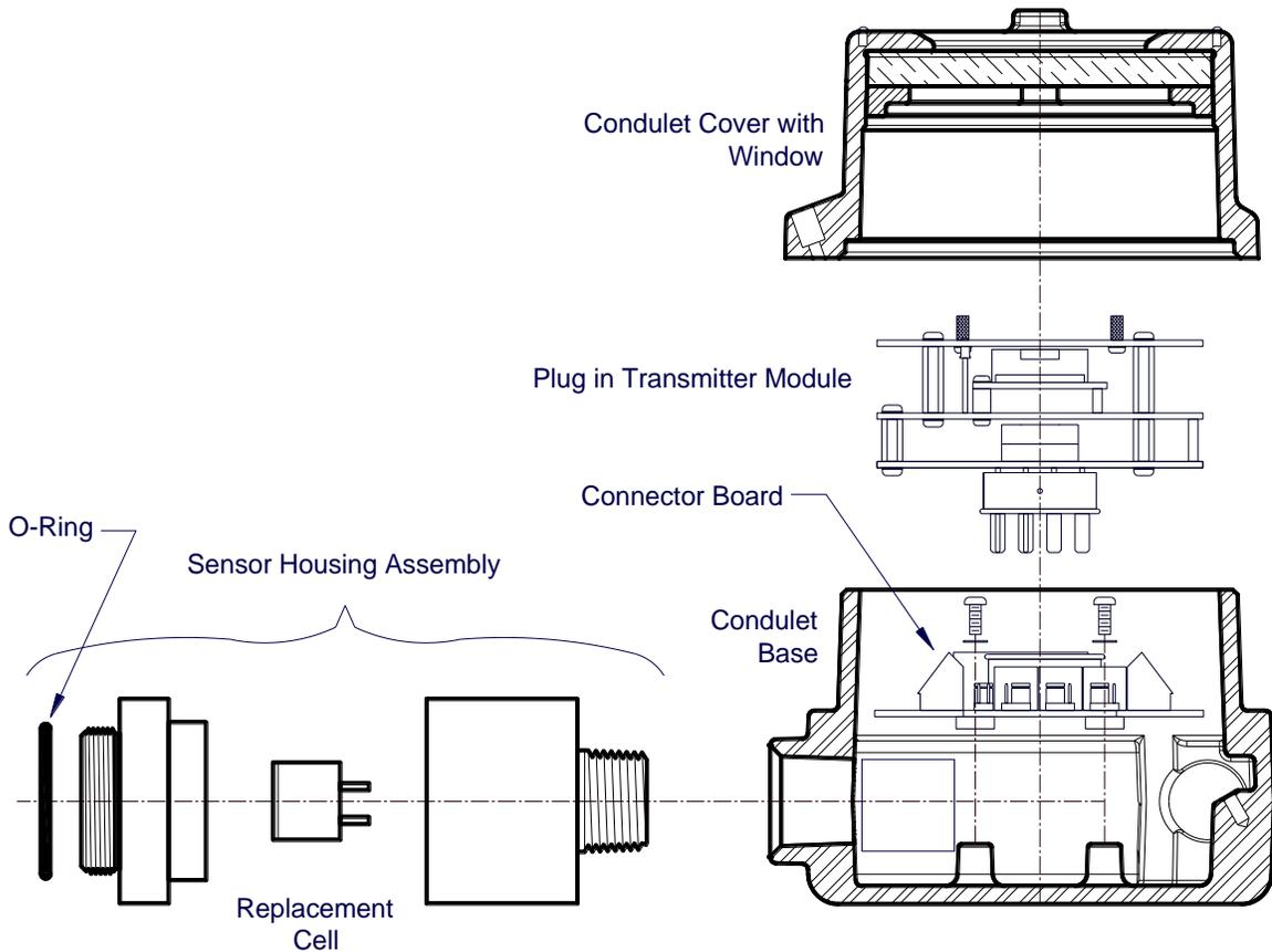
**Figure 16** IR-640/IR-642 Replacement Parts
