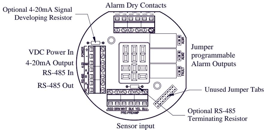
Figure 7 Connector Board Terminals
