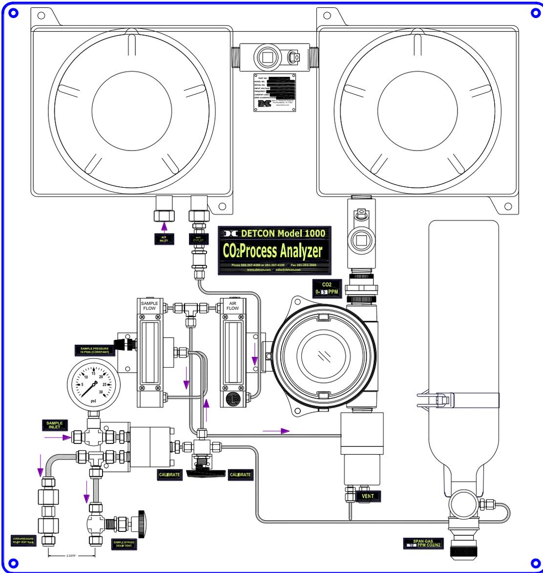
Figure 18 Unit Flow Diagram
