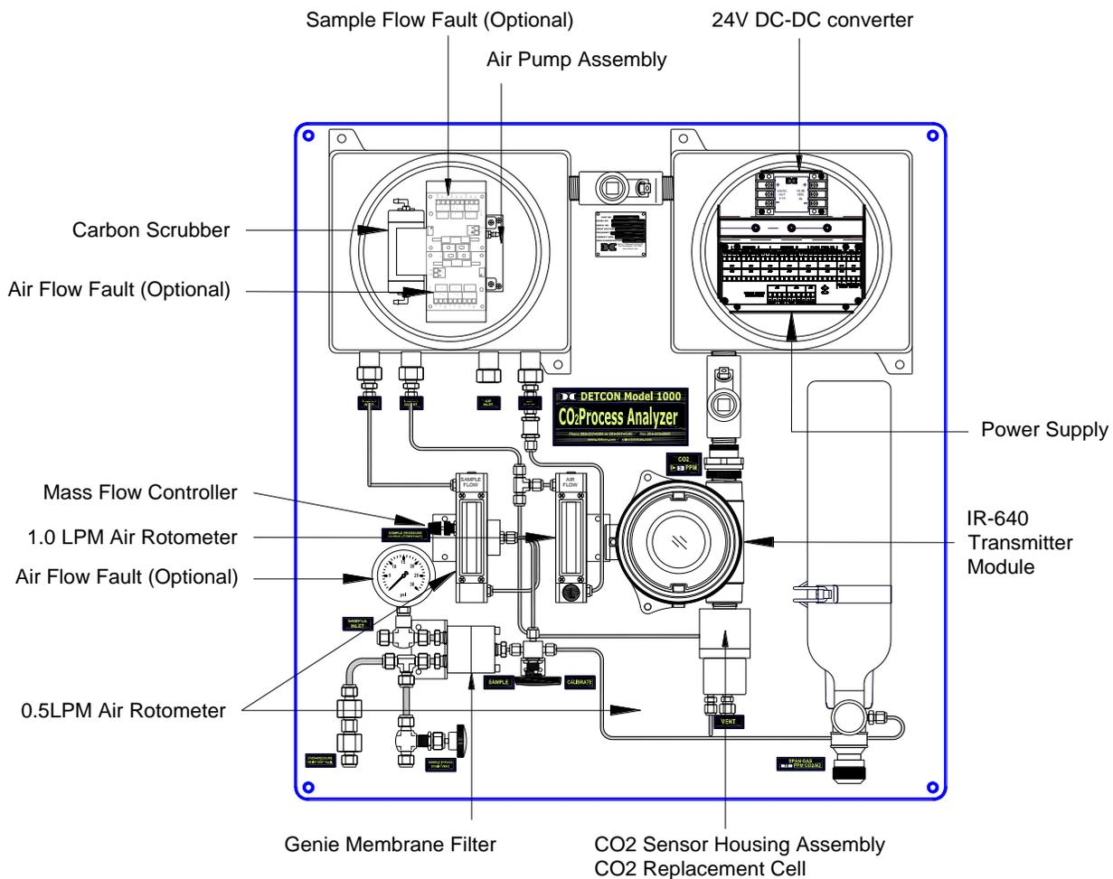
**Figure 17** Analyzer Spare Parts
