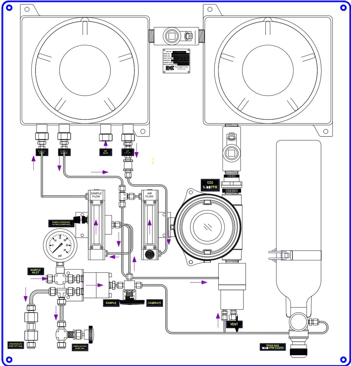
Figure 19 Unit Flow Diagram with Flow Fault
