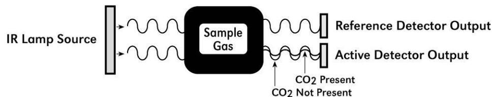
Figure 4 Principle of operation
