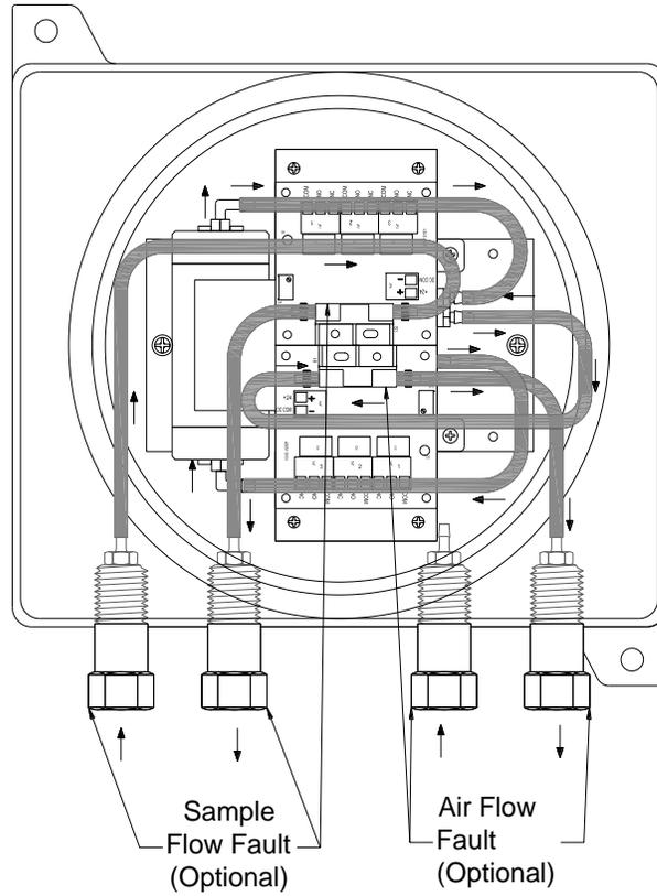
**Figure 20** Pump Box Flow Diagram
