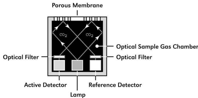
Figure 2 Sensor Diagram
