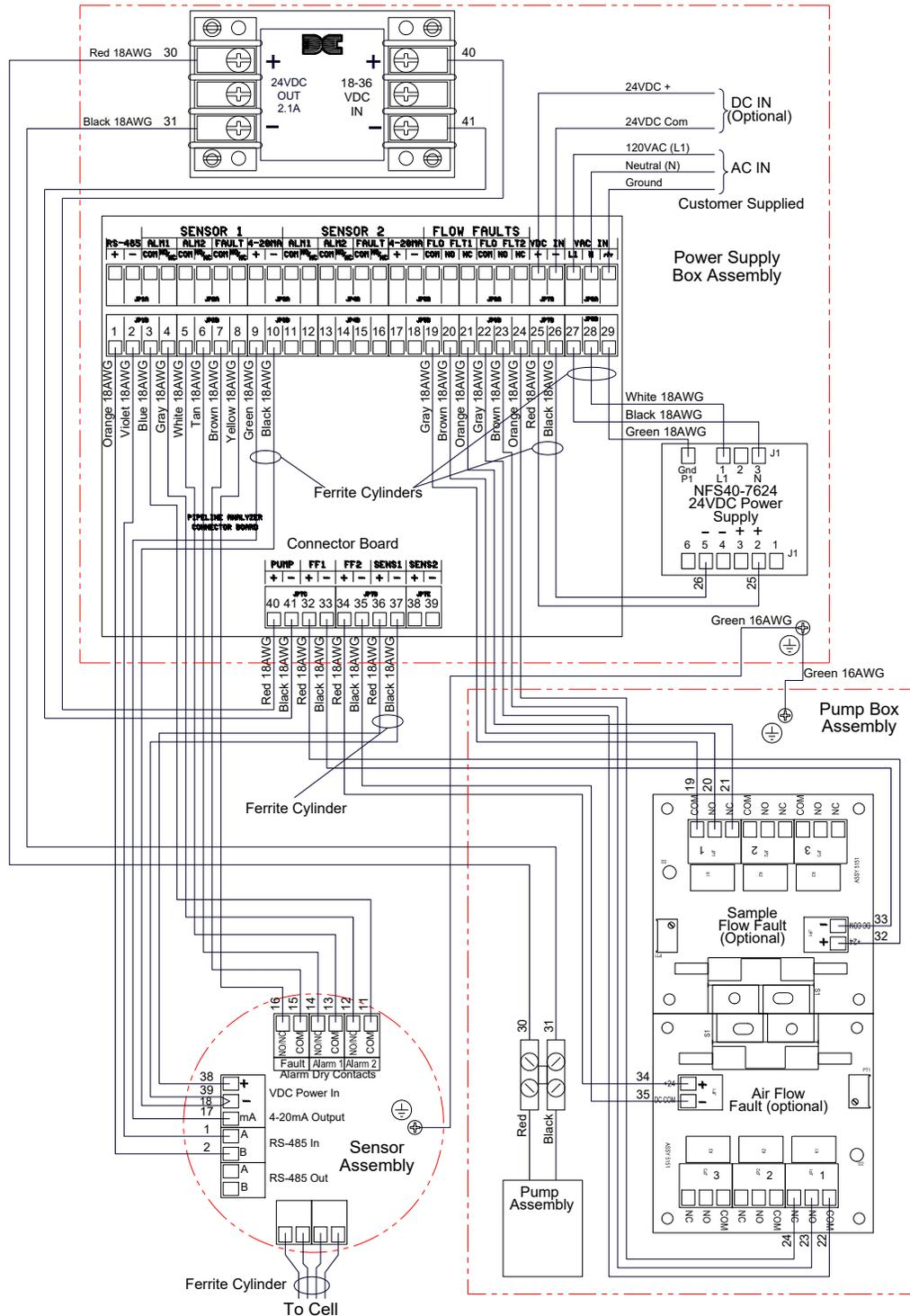
**Figure 21** Wiring Diagram
