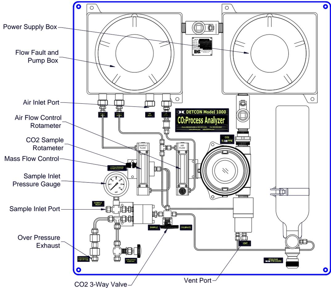
**Figure 10** Unit Overview (Ir-640 0-15% with Air Dilution shown)
