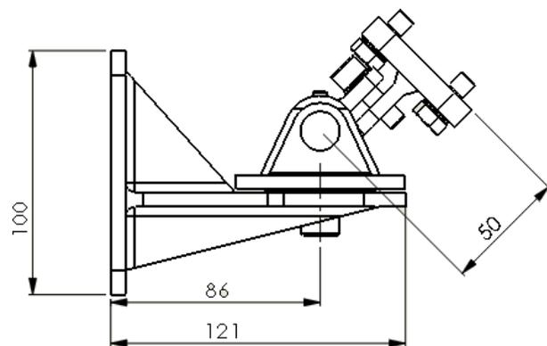
Figure 12 : Tilt mount base – Side View
