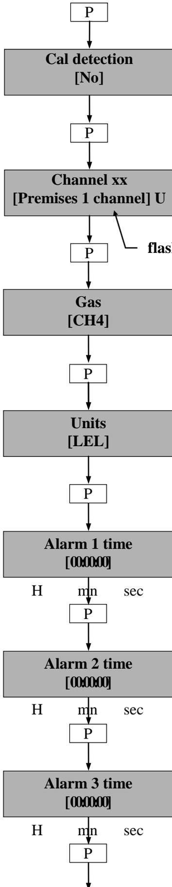
The MX52 unit can detect and indicate (with a flashing yellow LED) that a line has been placed in CALIBRATION mode on the detector.
