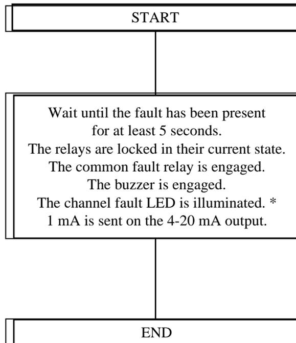
\* The LED is extinguished as soon a the fault disappears.
