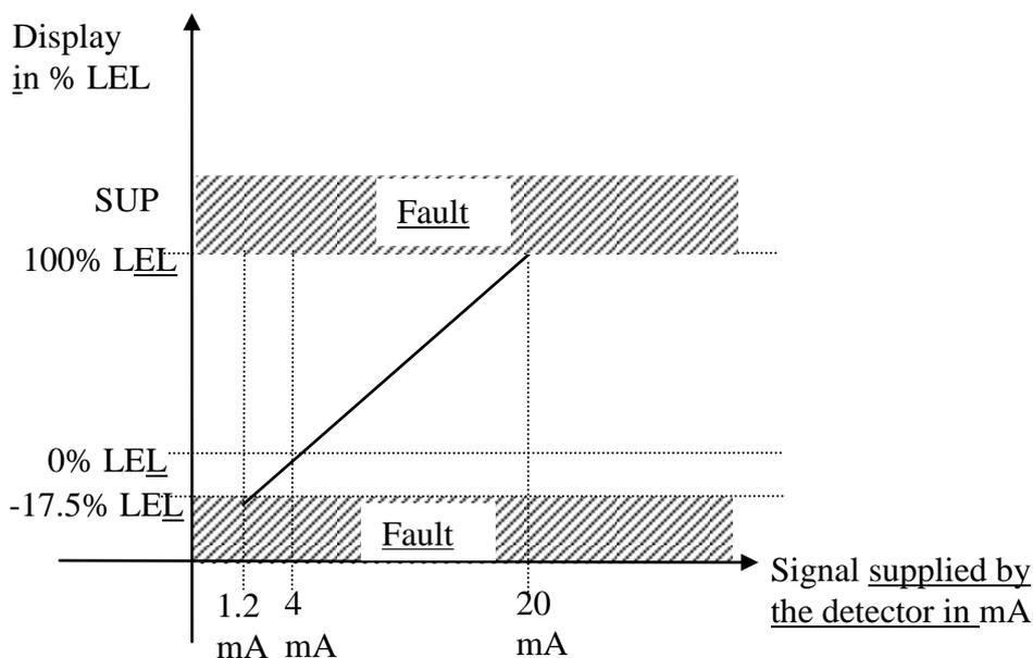
**Please note:** When the value measured is  $\geq 100\%$  LEL, the measuring device memorises the fact that the value has exceeded the scale and the channels switch to alarm and fault mode. Resetting these statuses is a manual operation to be performed by the user, who must follow the safety regulations specific to the site. The reset is checked either by turning the device on and off or by a maintenance inspection.
