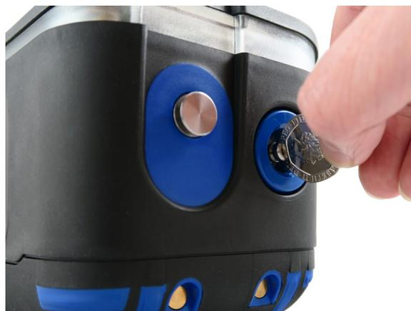
**Figure 70: Inlet Nozzle Removal**
