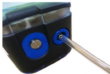
**Figure 87: Connect Calibration Gas**
