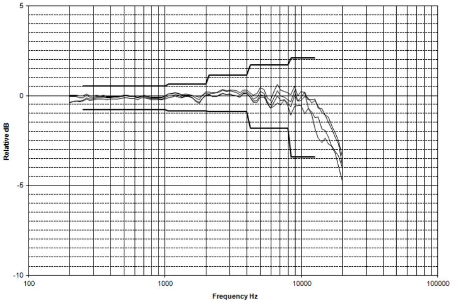
**Directional frequency response using windscreen & remote preamp (0°-90° incidence angles)**
