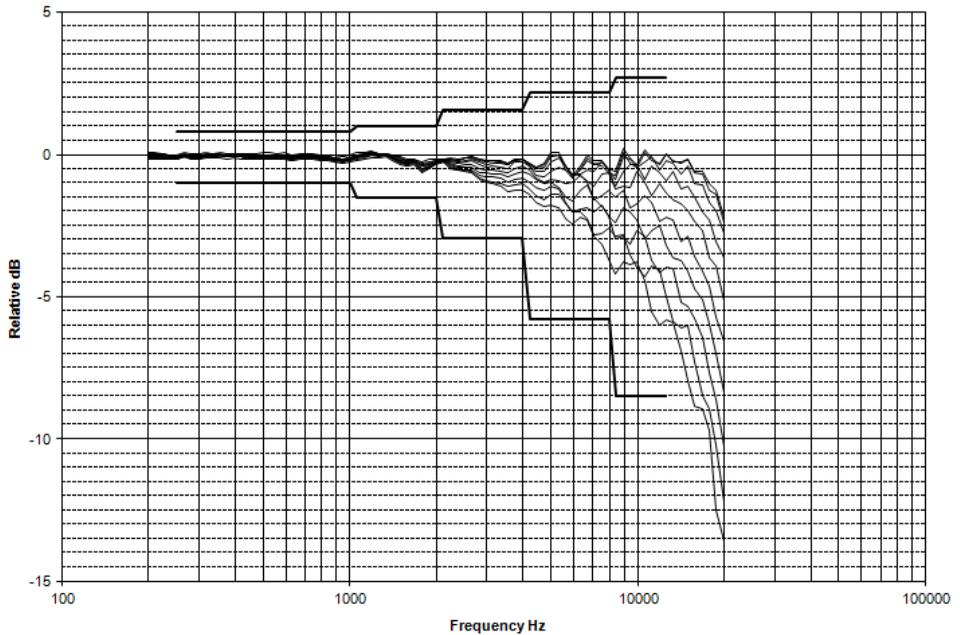
**Directional frequency response positioned with a remote preamp (0°-150° incidence angles)**
