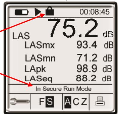
Figure 3-9: Secure run and measurement screen
