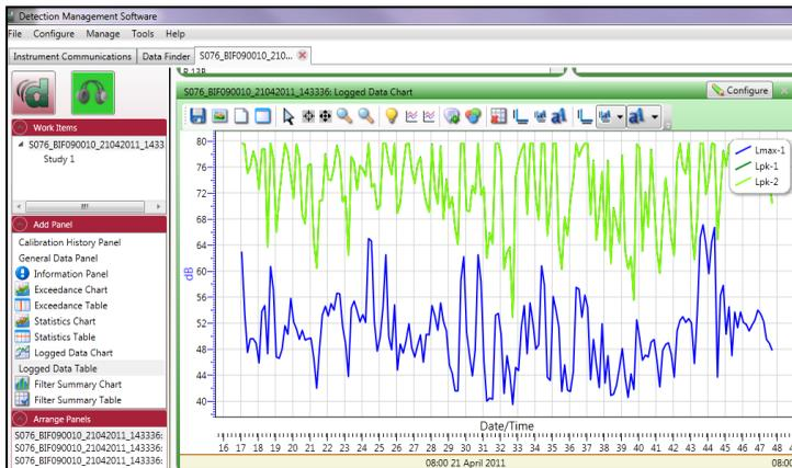
Figure 1-3: Acoustic data and DMS charting example
