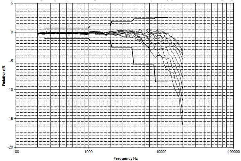
**Directional frequency response using windscreen & remote preamp (0°-150° incidence angles)**
