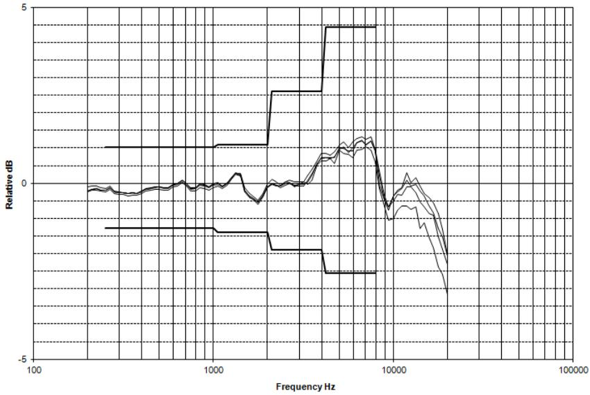
**Directional frequency positioned side toward noise source (0°-90° incidence angles)**
