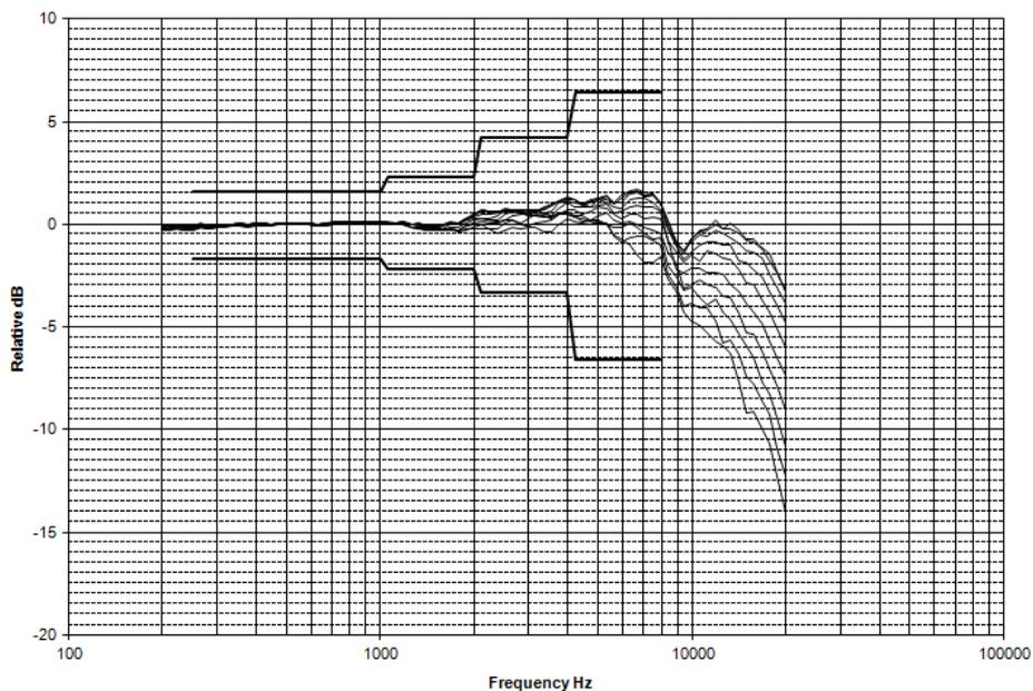
**Directional frequency response positioned side noise source (0°-150° incidence angles)**
