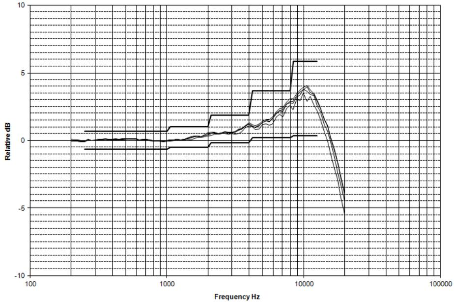
**Directional frequency response positioned back toward noise source (0°-90° incidence angles)**
