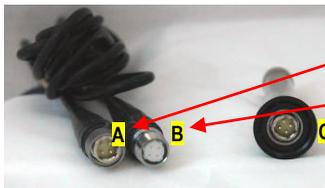
Extension cable with connector pins (see **A**) connects to the top of the SE-400.
