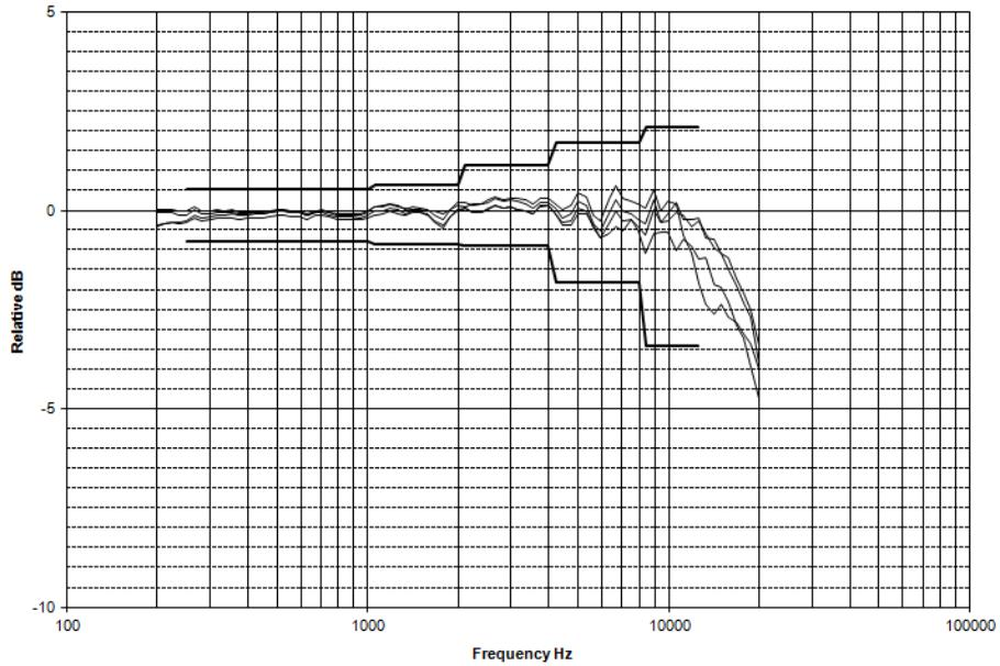
**Directional frequency response positioned toward noise source (0°-90° incidence angles)**
