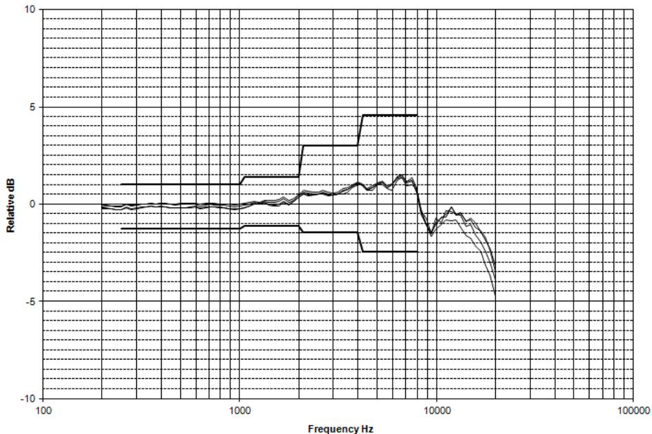
**Directional frequency response positioned facing toward noise source (0°-90° incidence angles)**
