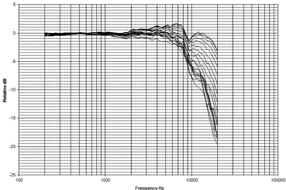
**Directional frequency response positioned side noise source (0°-90° incidence angles)**
