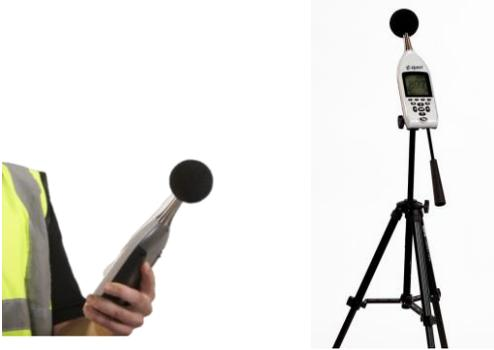
Figure 4-7: Measurement positioning and tripod mount
