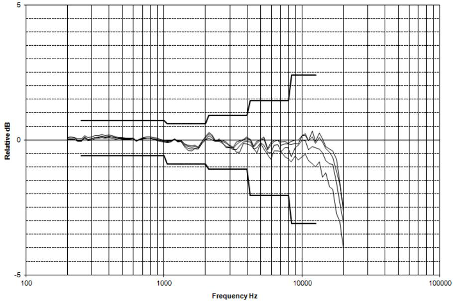
**Directional frequency response positioned side toward noise source (0°-90° incidence angles)**
