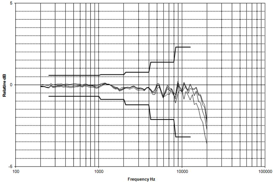
**Directional frequency response positioned with a remote preamp (0°-90° incidence angles)**
