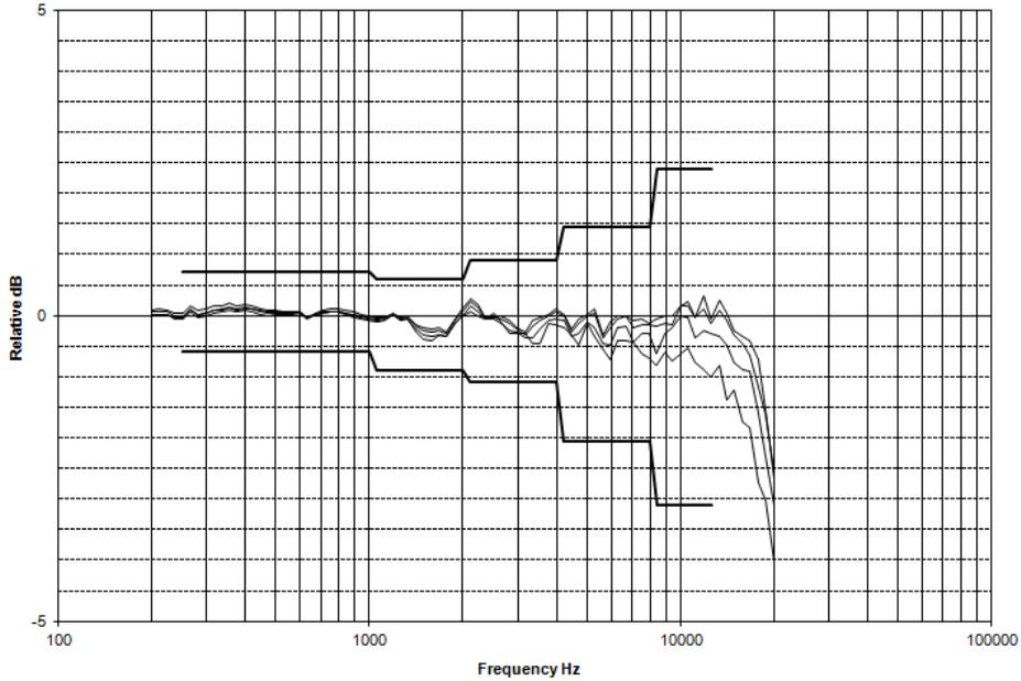
**Directional frequency response positioned with side toward noise source (0°-90° incidence angles)**
