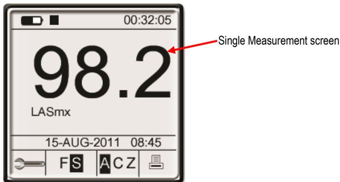
Figure 4-9: Single measurement screen in stop mode
