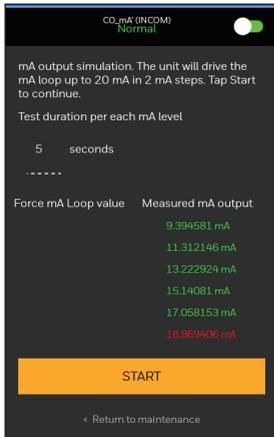
To perform a full range test of the mA loop, use the mA Loop Simulation feature.
