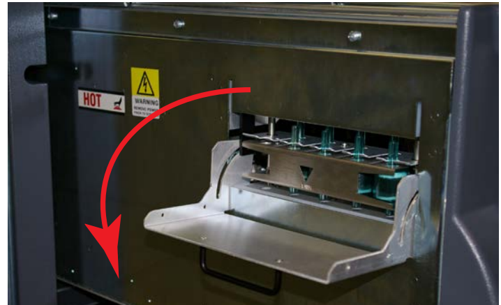
Figure 5-5. Pyrolyzer Filter Door
