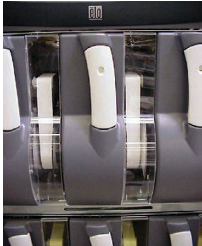
Hook front of keyboard tray into slot under first tier of analyzers.
