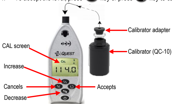
Figure 1-10: Calibrating the SD-200
