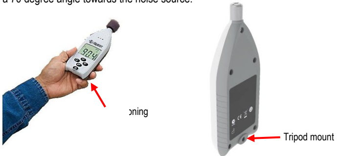
Figure 1-9: Positioning and tripod mount
