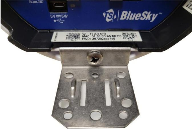
**Figure 17:** Mounting bracket
