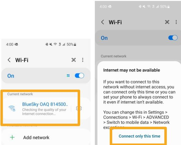
**Figure 10:** Manually connect to Wi-Fi®
