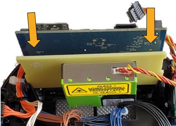
**Figure 37:** Install new sensor
