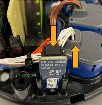
**Figure 43:** Disconnect sensor cable
