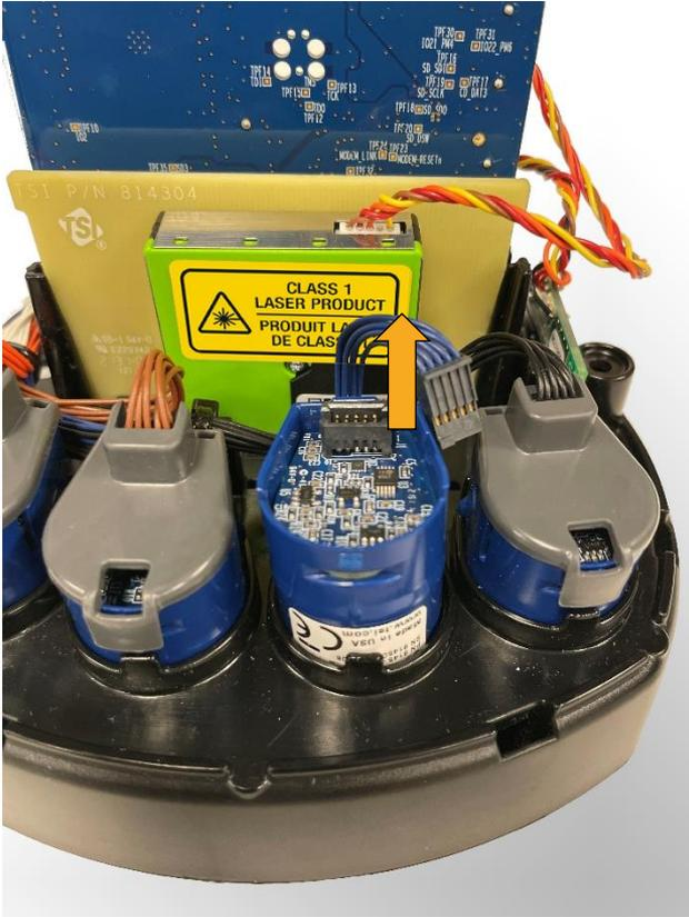
**Figure 39:** Disconnect sensor cable
