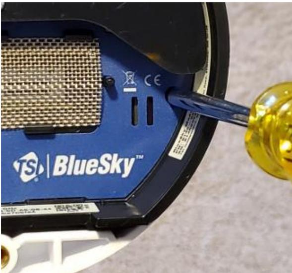
**Figure 34:** Remove cover screws
