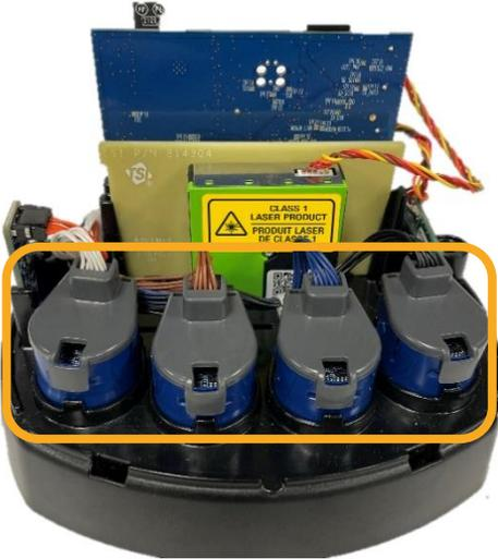
**Figure 38:** Replace electrochemical sensors
