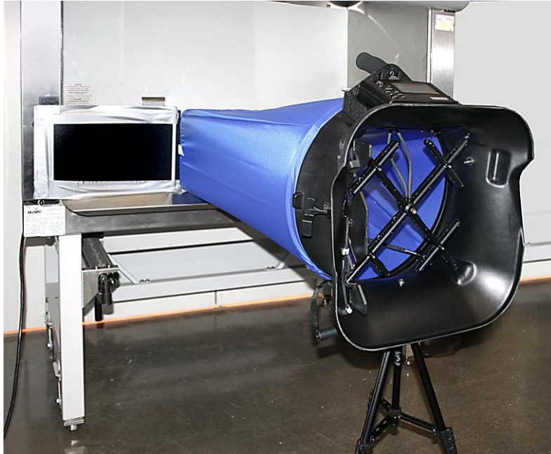
Figure 28: Adjust Height and Position of Telescopic Stand
