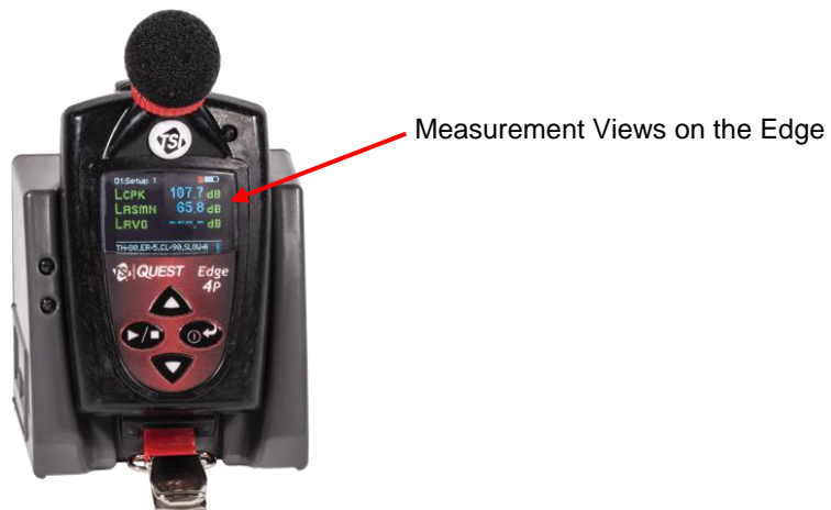
Figure 4-9 Measurement View on the Edge
