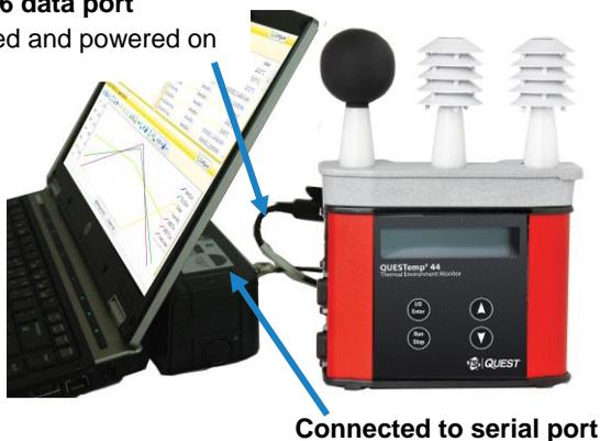
Figure 30: Communicating with the QT<sup>o</sup> 44/46 and DMS
