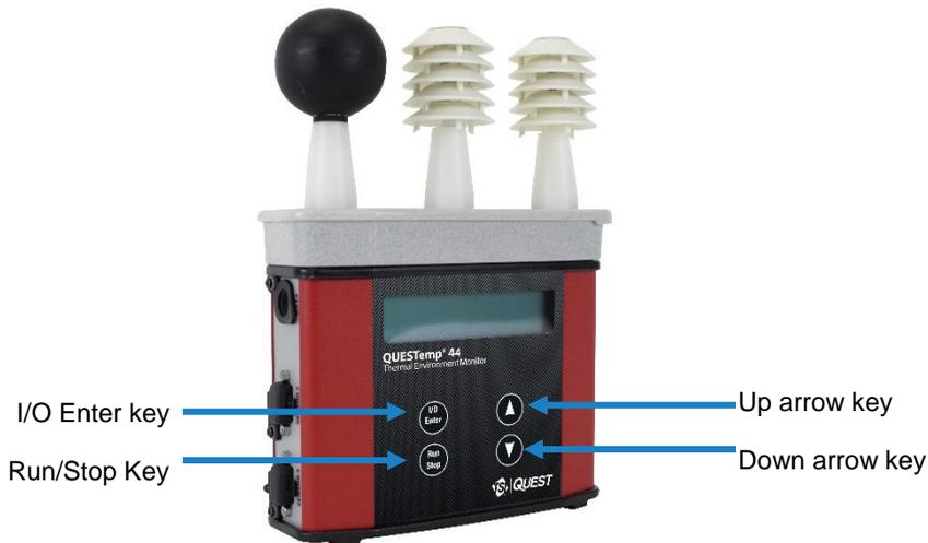
Figure 2: Keypad explained and identified
