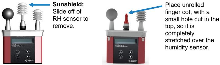
**Figure 22: Sunshield & placement of finger cot prior to RH verification**
