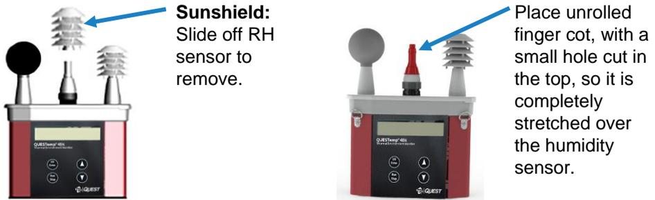
**Figure 26: Sunshield and placement of finger cot prior to RH alignment**
