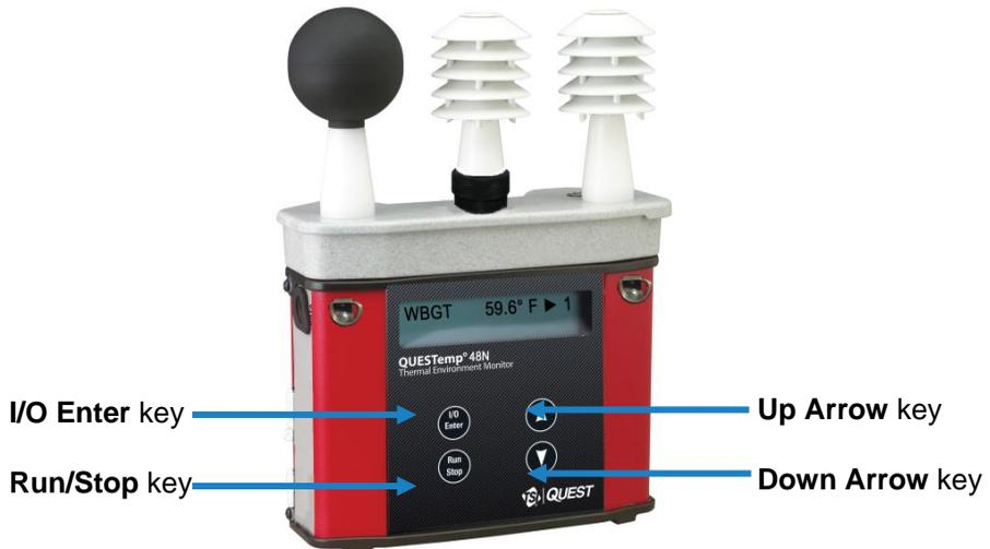
**Figure 2: Keypad Keys identified**
