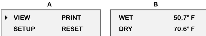
Figure 24: Main menu with view selected (A) & measurement screen (B)
