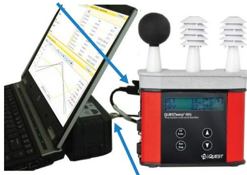
Connected to serial port
