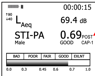
Figure 6-27: Post CAP-1 applied during STI-PA test
