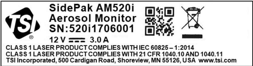
There are no user-serviceable parts inside this instrument. Performing services other than those described in this manual may result in exposure to harmful (visible) laser radiation. A warning label like the one shown below is affixed to the internal laser device.
