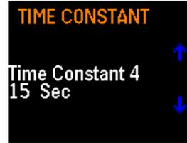
The SidePak™ AM520/AM520i always makes a measurement once every second and updates the display every second regardless of the Time Constant selected. Using a Time Constant greater than one second results in displayed readings that are averages of the 1-second readings. For example, a 10-second Time Constant will cause the display to show an average of the most recent ten 1-second readings. In other words it is a 10-second "moving average," updated every second.
