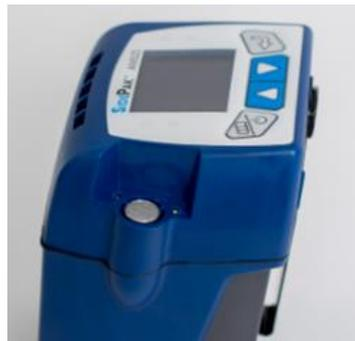
6. Place inlet gasket on the inlet so that the tabs on the gasket fit inside the inlet around inner tabs of the inlet as shown.
