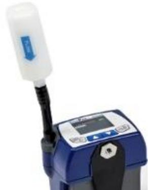
6. The instrument will count-down from 60 to 0 and display Zero Cal Complete.
