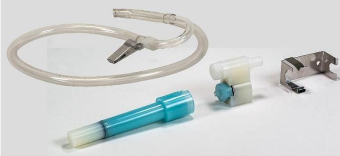
The DPM cyclone is designed with a 50 percent cut-off size of  $0.8 \mu\text{m}$ . The Dorr-Oliver cyclone is positioned upstream of the DPM cyclone to filter out particles larger than  $4 \mu\text{m}$  preventing large particles from clogging the inlet of the DPM cyclone.
