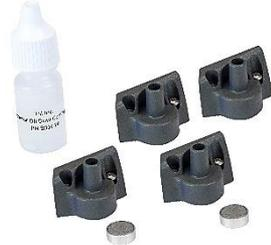
The “standard inlet” does not have a size marking on the top edge and does not cause any specific particle size separations. It is intended for use with external size-selective aerosol samplers such as a cyclone or external impactor at any flow rate within the allowable range. When using a cyclone or external impactor, the impactor disk should not be used.
