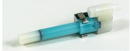
3. Attach the DPM cyclone assembly and sample tube onto the inlet.
