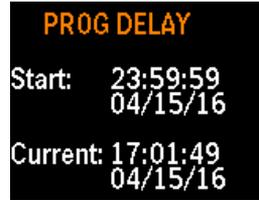
Program logging mode uses start and stop time/date, logging interval, test length, number of tests, and wait time between tests programmed in using TrakPro™ software. If the aerosol Response Concentration feature is enabled (set in the “**Response Conc**” option of the **SETTINGS** menu), the logged data file will include both mass concentration and response concentration.
