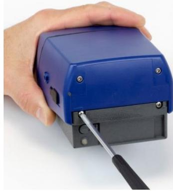
2. Firmly grip sides of instrument and sides of battery.
