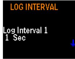
The SidePak™ AM520/AM520i always makes a measurement once every second regardless of the log interval selected. Using a log interval greater than one second results in stored data points that are averages of the 1-second readings. For example, a 10-second log interval will result in one stored data point every 10 seconds. Each of those data points will represent the computed average of ten, 1-second readings.
