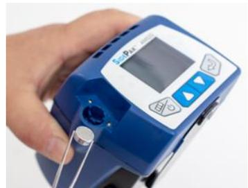
3. Clean the impactor inlet and impactor disk with a clean lint-free swab or microfiber cloth and light solvent. Gently blow impactor body dry with canned/pressurized clean air or allow to air dry. Use a lint-free swab or microfiber cloth to clean impactor well inside the instrument case to remove accumulated particles.
