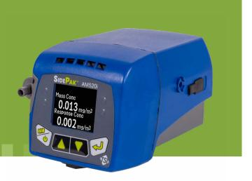
The SidePak™ AM520i Personal Aerosol Monitors are small, portable, battery-operated, data-logging, light-scattering laser photometers that provide real-time aerosol mass concentration readings of dusts, fumes, mists, smoke and fog within a worker breathing zone.
