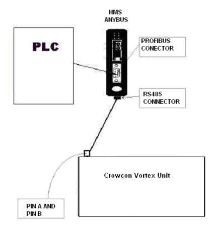
The next section explains exactly which PINs should be connected from the HMS AnyBus device to the Crowcon Vortex unit.
