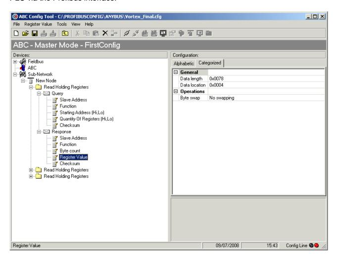
Other Read Holding Registers requests read the alarm data from later registers in the Vortex unit and store them directly after the channel analogues data in its internal registers. This makes it easier for the Profibus to read this data as a single block.
