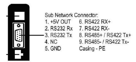
The AnyBus female 9 way cannon "D" connector (Sub Network Connector) shown above should be connected to the Vortex Node Controller Module as follows:
