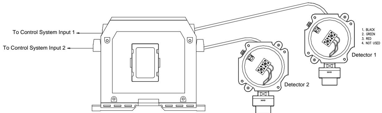
Connect the positive, signal and negative terminals of the detector(s) to the corresponding terminals of the appropriate input channels on the mV Bridge Converter Module (see diagram). The module terminals are arranged as follows:
