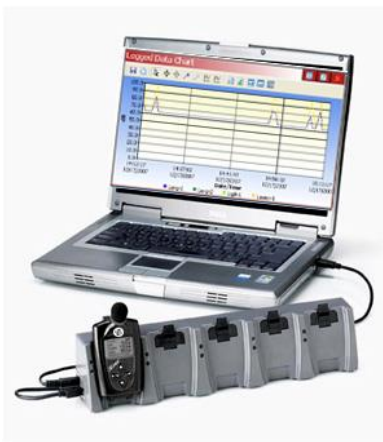
Figure 5-1: Communicating between your PC and the Edge
