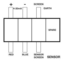
The unit requires a nominal 18 to 30V, 30m current-loop-powered supply.
