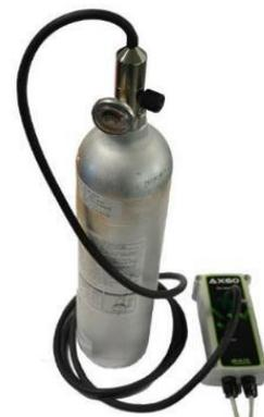
**Step 4]** Fit the regulator to the check gas bottle
