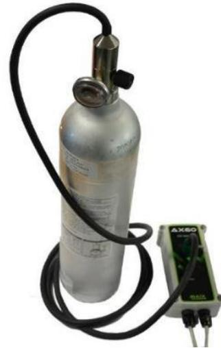
**Step [4] Fit the regulator to the 1.6% CO<sub>2</sub> gas bottle**
