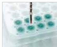
This pH electrode with temperature compensation sensor can take measurements from samples as small as 50 $\mu$ L, the smallest in the world.
