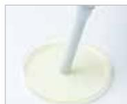
The sensor is located on the flat surface of the electrode tip, with less than a 100  $\mu$ m protrusion from the housing.
