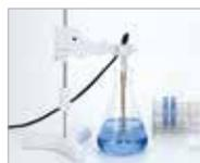
283 mm length & 8 mm diameter. The long, thin design makes this electrode perfect for measuring in large containers and test tubes.
