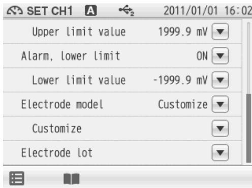
1. Tap  on the right of the Electrode model item. The electrode model selection screen appears. Tap  when do not reflect the setting.
