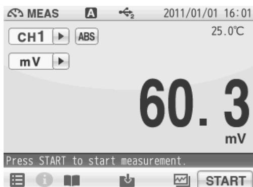
1. Tap the channel setting and the measurement item in the MEAS screen to set "CH1" and "mV".
