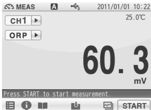
1. Tap the channel setting and the measurement item in the MEAS screen to set "CH1" and "ORP".
