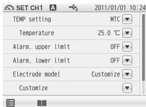
1. Display the Temperature item when select MTC. Tap
