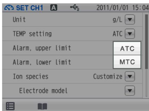
There are two types of temperature compensation for ION measurement; Automatic Temperature Compensation (ATC) and Manual Temperature Compensation (MTC).
