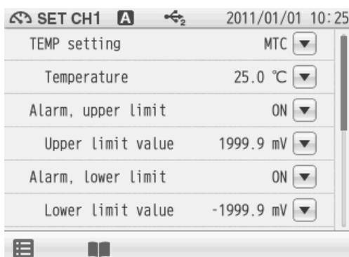
1. When selecting ON the Alarm, lower limit item, the Lower limit value, tap  on the right of the Lower limit value item.
