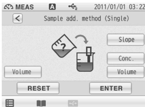
1. Tap **>** on the right of the Sample addition method item in the ION standard addition mode screen.
