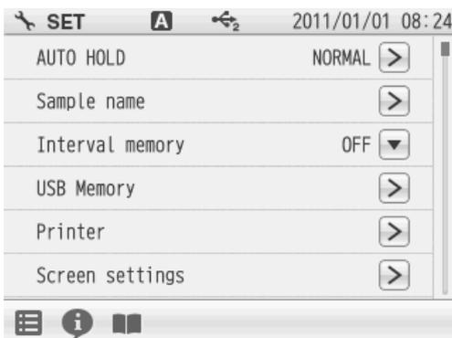
In the AUTO HOLD mode, the instrument judges potential stability automatically to the measurement values. This instrument allows you to select one among the 6 type criteria of potential stability.
