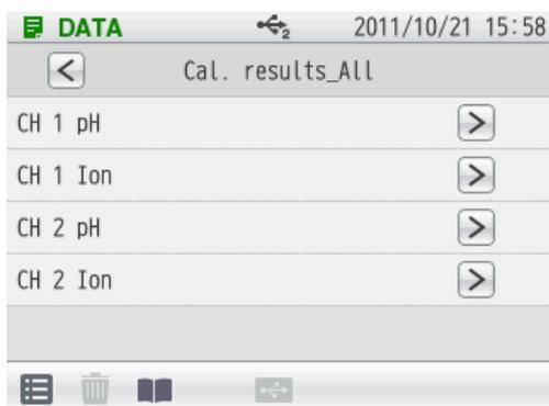
You can check the latest 20 data of pH and ION calibration.
