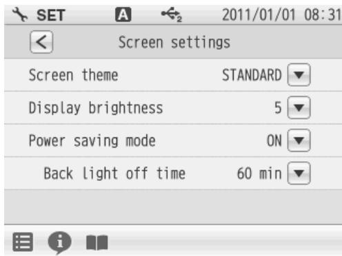
When selecting ON for Power saving mode, the Back light off time item is displayed.
