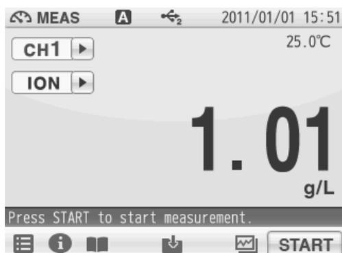
1. Tap the channel setting and the measurement item in the MEAS screen to set "CH1" and "ION".
