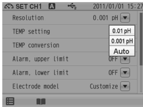
You can switch the resolution for pH measurement values to 0.01 pH, 0.001 pH, or Auto. If Auto is set, the resolution is switched automatically to 0.001 pH when the variation of pH measurement value is 0.01 pH or less in the latest 10 seconds, to 0.01 pH for the rest. This is a convenient function to judge the stability of pH measurement values.
