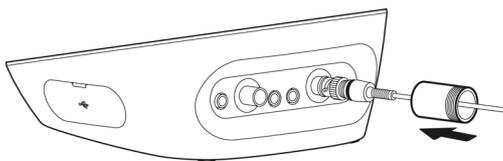
1. Insert the groove of electrode connector by fitting with the connector socket pin of the instrument.
