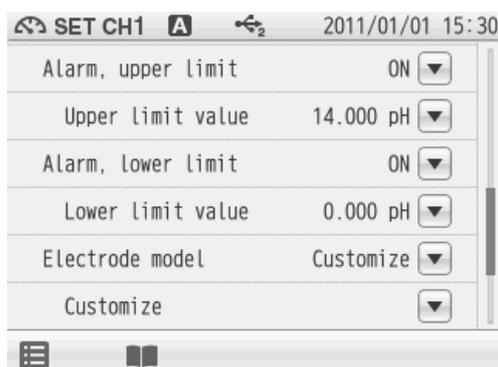
1. When selecting ON the Alarm, lower limit item, the Lower limit value, tap
