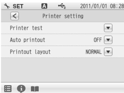
When a printer is connected with the instrument, this item allows you to perform a printer test.
