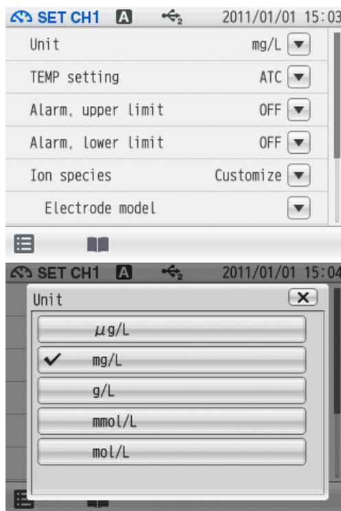
You can select  $\mu\text{g/L}$ ,  $\text{mg/L}$ ,  $\text{g/L}$ ,  $\text{mmol/L}$  or  $\text{mol/L}$  as the ION measurement unit.
