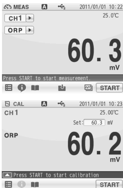
1. Tap the channel setting and the measurement item in the MEAS screen to set "CH1" and "ORP".
