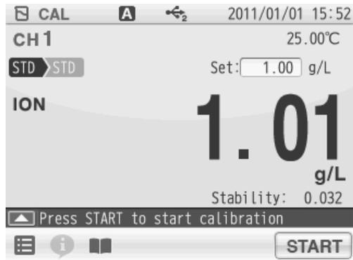
1. Tap the ION value at the right of "Set:" to display the numerical-key screen.
