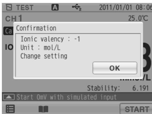
Follow the guidance to calibrate the instrument by simulated input of 0 mV and 120 mV in the order below and check the following operation.
