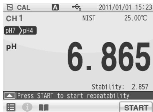
1. When calibration for all of the points is completed, the repeatability is automatically checked.
