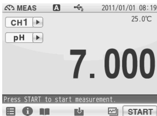
1. Tap the channel setting and the measurement item in the MEAS screen to set "CH1" and "pH".
