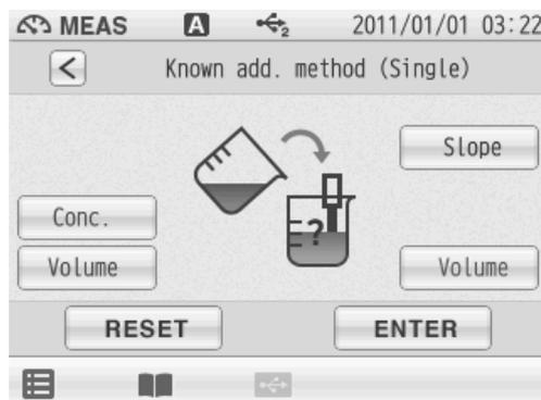
1. Tap  on the right of the known addition method item in the ION standard addition mode screen.
