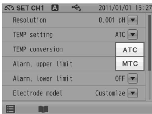
There are two types of temperature compensation for pH measurement; Automatic Temperature Compensation (ATC) and Manual Temperature Compensation (MTC).
