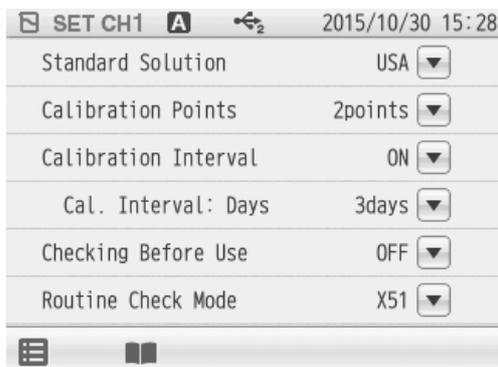
1. Display the Cal. Interval item when select ON at the calibration interval. Tap  on the right of the Cal. Interval item.
