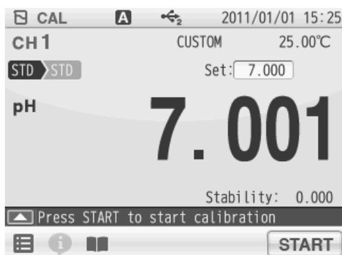
1. Press the CAL key to display the pH CAL screen.
