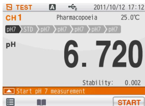
1. Immerse the pH electrode in the standard solution, and tap **START** to start measurement.
