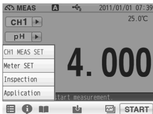
In the known addition method (Single), the targeted ion concentration in a sample solution is obtained from a change in electric potential by adding once a small amount of the target ion solution to the sample solution.
