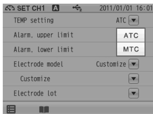
There are two types of temperature setting for mV measurement; Automatic Temperature setting (ATC) and Manual Temperature setting (MTC). In ATC, the instrument detects the solution temperature with the connected temperature sensor, and displays it on the screen. In MTC, measure the solution temperature and enter the value in advance. The instrument displays the entered temperature.
