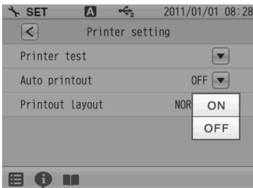
When a printer is connected with the instrument, this item allows you to perform an automatic printer test after measurement or calibration completion.
