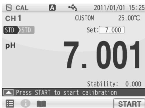
1. Tap the pH value at the right of "Set:" to display the numerical-key screen.
