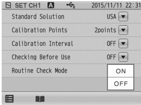
If you set the Checking Before Use setting to ON, it allows you to check repeatability after calibration by comparing the measured value of pH7 standard solution with the calibration result. After the set point calibrations are completed, repeatability is automatically checked using the deviation between the calibrated and measured values at pH7.
