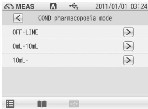
This is the test procedure for purified water, sterile purified water or water for injection contained in a container of 10 mL or less. The value when the measured temperature is at  $25^{\circ}\text{C} \pm 1^{\circ}\text{C}$  and the conductivity change for 5 minutes is  $0.1 \mu\text{S}/\text{cm}$  or less is judged whether it exceeds the evaluation standard,  $25 \mu\text{S}/\text{cm}$  or not.
