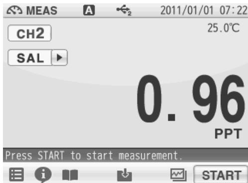
1. Tap the channel setting and the measurement item in the MEAS screen to set "CH2" and "SAL".
