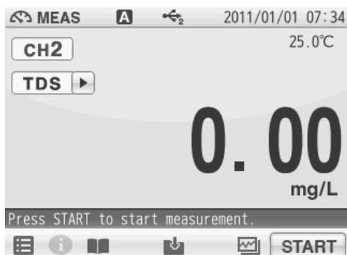
1. Tap the channel setting and the measurement item in the MEAS screen to set "CH2" and "TDS".
