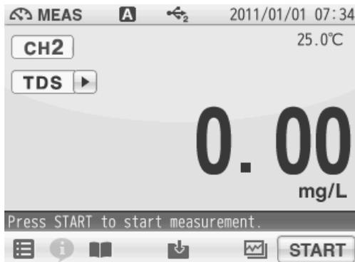
1. Press the MEAS key, and tap the channel setting and the measurement item in the MEAS screen to set "CH2" and "TDS".
