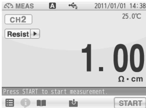
1. Press the MEAS key, and tap the channel setting and the measurement item in the MEAS screen to set "CH2" and "Resist".
