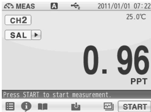
1. Tap the channel setting and measurement item in the measurement screen to set "CH2" and "SAL".
