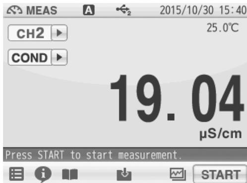
1. Press the MEAS key, and tap the channel setting and the measurement item in the MEAS screen to set "CH2" and "COND".
