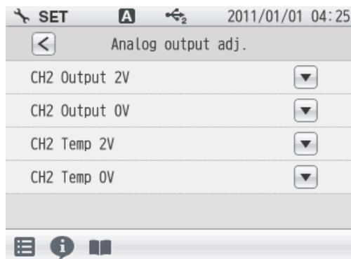
Connect the instrument with a digital multimeter, digital recorder, pen recorder or the like using a designated cable (analog output cable: Parts No.3014030152), and check and adjust the analog output value of the instrument.
