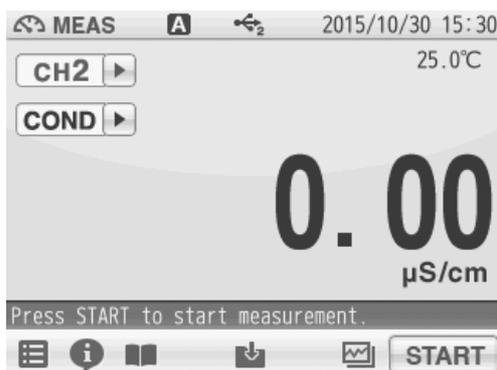
1. Tap the channel setting and the measurement item in the MEAS screen to set "CH2" and "COND".
