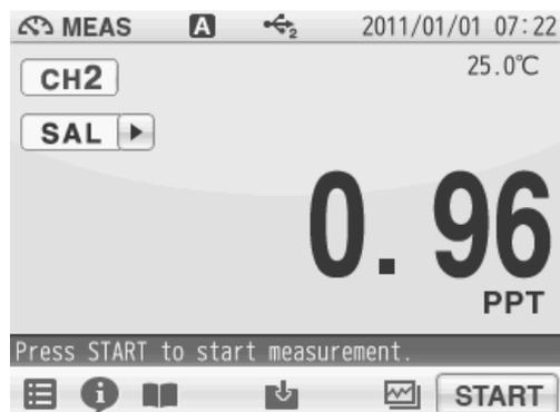
1. Press the MEAS key, and tap the channel setting and the measurement item in the MEAS screen to set "CH2" and "SAL".
