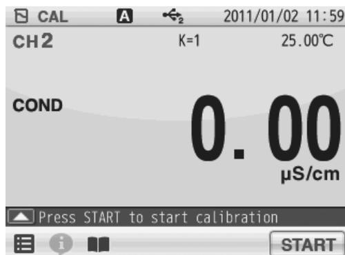
1. Tap the channel and measurement item in the measurement screen to set "CH2" and "COND".
