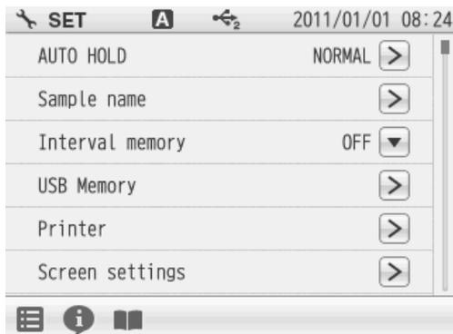
The Printer item allows you to set printing contents, etc. effective only when a printer is connected with the instrument.
