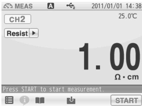
1. Tap the channel setting and the measurement item in the MEAS screen to set "CH2" and "Resist".
