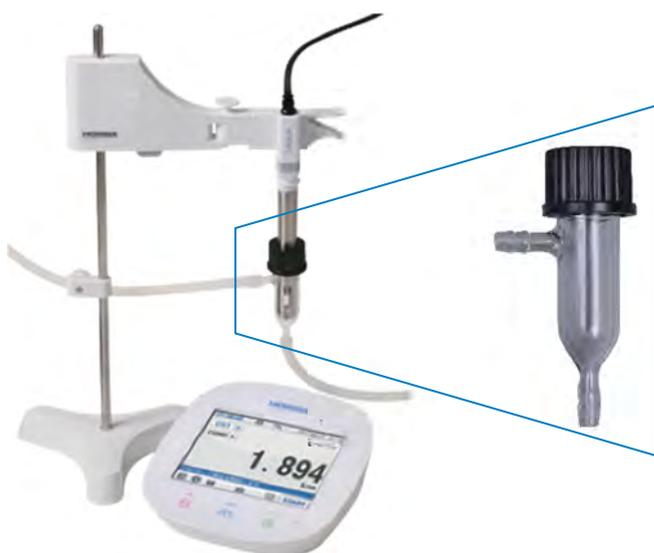
Use the flow cell in combination with the 9371-10 stainless steel conductivity cell to measure ultra-pure water.
