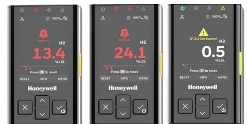
Alarm 1 state Alarm 2 state Fault state
