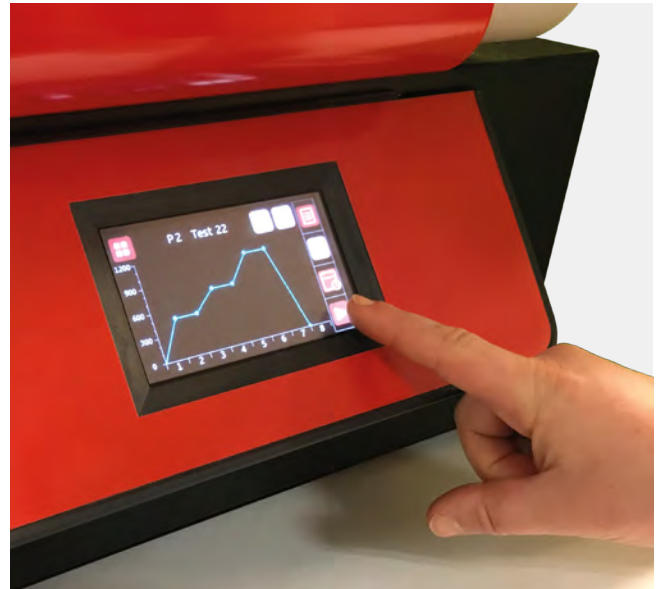
The CC-T1 touch screen controller in use.
