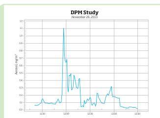
Time History – Graphically displayed, logged data can display high and low exposure concentrations that cannot be identified with traditional gravimetric sampling. This example of actual customer data illustrates the value of seeing what time peak exposure occurred. This enables an industrial hygienist to investigate the cause of the spike at 12:00 and recommend corrective actions specific to the cause of the exposure without delay.
