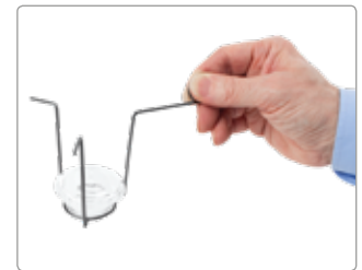
Wire crucible holder (standard) with crucible and lid (optional)
