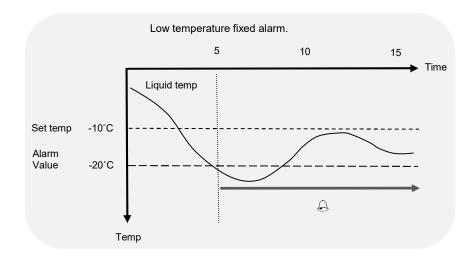
3. A hold-off time can be entered, which is a user adjustable time of between 0 and 21mins for which the alarms remain muted after either button has been pressed to acknowledge an alarm condition. If the bath returns to the value such that the alarm level is not exceeded the alarm will cancel. However, if the temperature remains outside the alarm level the alarm condition will re-occur after this hold-off time.
