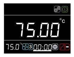
1. Rotate the dial until the **countdown timer** icon is highlighted, press the **S** button.
