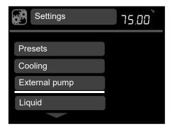
2. Rotate the dial to scroll up and down the list, until **External pump** is highlighted, press the **S** to select.
