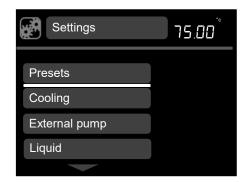
2. Rotate the dial to scroll up and down the list, until **preset** is highlighted, press the **S** to select.
