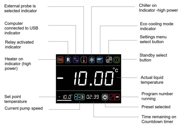
Navigation around the home screen is achieved by rotating the main dial which moves a white cursor to highlight function icons. Pressing the **S** button whilst the icon is highlighted will change the colour of the cursor to red, make the icon active and allow changes to be made, or in the case of the settings icon, further menus to be displayed. Press the **F** button to cancel an active icon. The cursor will then change to white.
