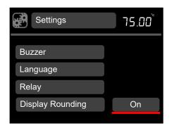
3. Rotate the dial to toggle between on and off, press **S** to save the selection.
