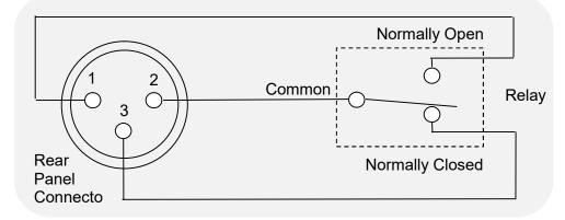
For the connecting cable use a mating XLR style connector such as the NC3FXX manufactured by Neutrik AG
