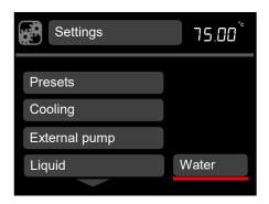
3. Rotate the dial to scroll through the liquid options, press **S** to save the selection.
