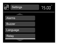
2. Rotate the dial to scroll up and down the list until **relay** is highlighted, press **S** to select.
