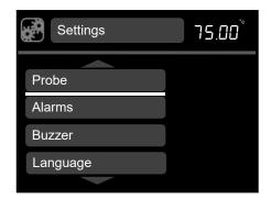
2. Rotate the dial to scroll up and down the list until **probe** is highlighted, press **S** to select.
