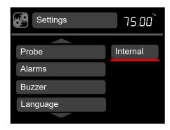
3. Rotate the dial to scroll through the probe types (external or internal), press **S** to save the selection
