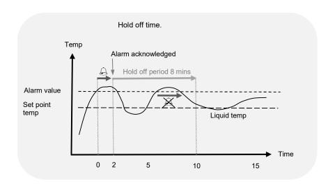
Each alarm can be programmed to latch, activate an audible buzzer and a relay. Alarms are cancelled by pressing the **F** or **S** button or if an alarm condition has been removed.
