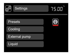
3. Rotate the dial to display preset icon 1, 2 or 3, press **S** to select.
