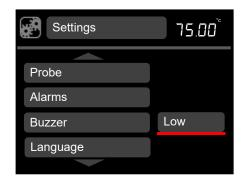
3. Rotate the dial to scroll through the volume levels (low, medium and high and off), press **S** to save the selection.
