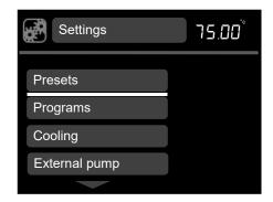
Rotate the dial to scroll up and down the list, until the desired setting is highlighted, press the S button to select. The desired settings menu is displayed.
