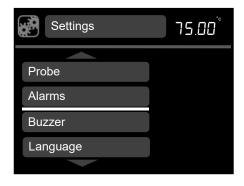
2. Rotate the dial to scroll up and down the list until **alarms** are highlighted, press **S** to select.
