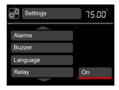
3. Rotate the dial to toggle between on/off, press **S** to save the selection.
