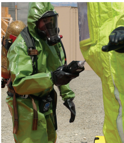
Workers can easily measure VOCs and wirelessly transmit readings up to 2 miles/3 km away.
