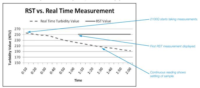
Although the sample continuously settles out of solution, the RST calculated value does not change.
