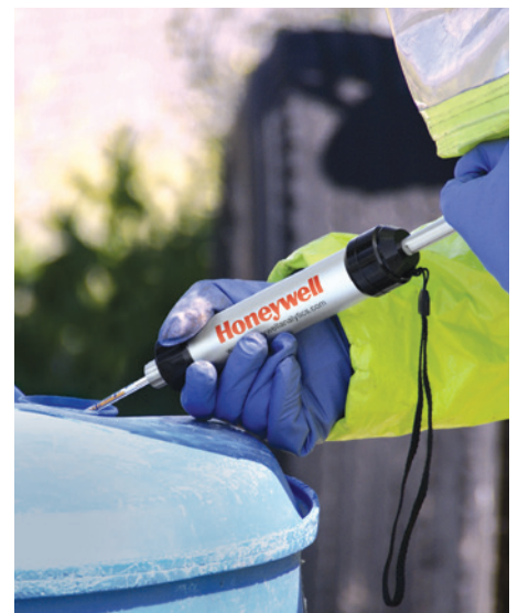
First responder uses Honeywell Colorimetric Tubes and Hand Pump to measure VOC levels inside a barrel.
