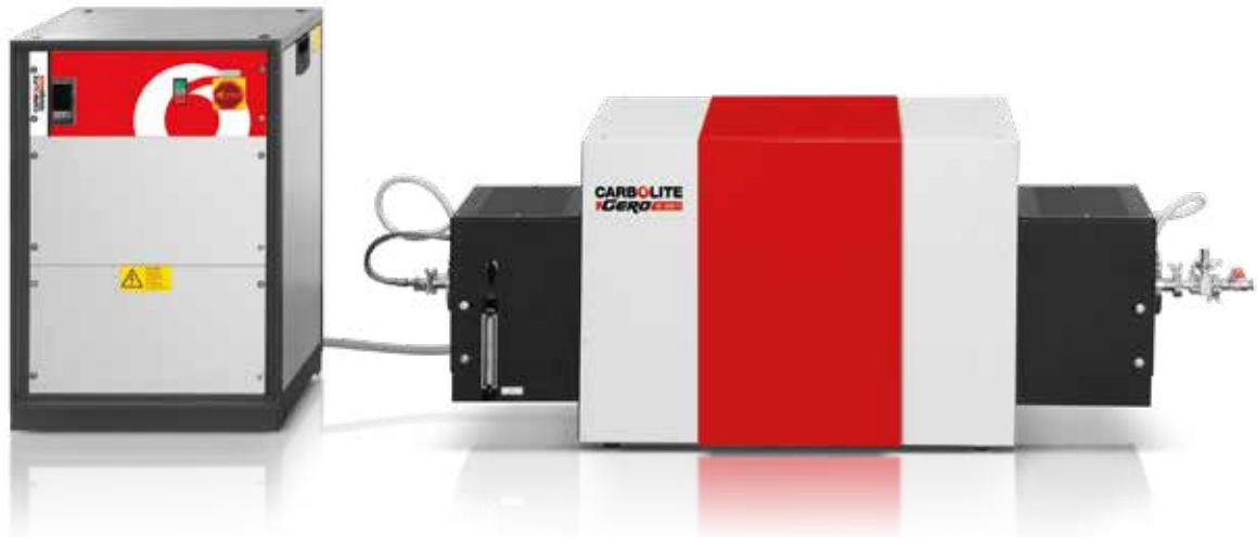
Horizontal High Temperature Tube Furnace HTRH 18/70/600 with optional EPC3008P10 programmer and optional high vacuum capable inert gas package (high vacuum capable up to 1450°C and up to 1800°C under normal pressure. Rotary vane pumps and turbo pumps optional available (see page 46).
