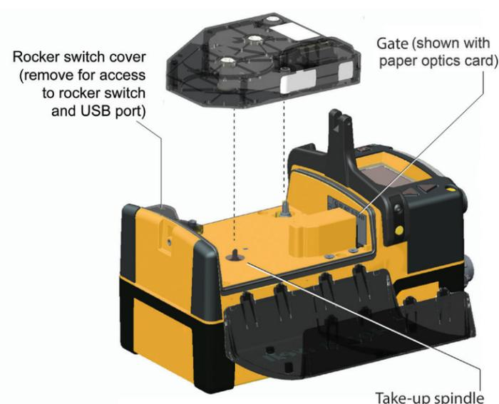
Figure 9: Loading a Chemcassette cartridge
