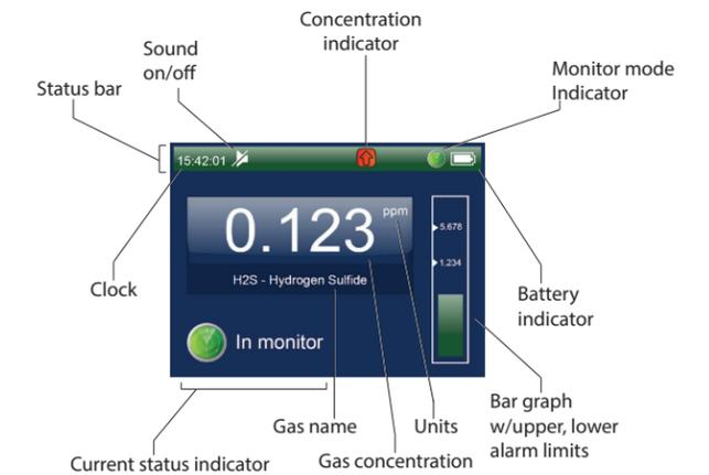
Figure 3: SPM Flex display - In Monitor mode
