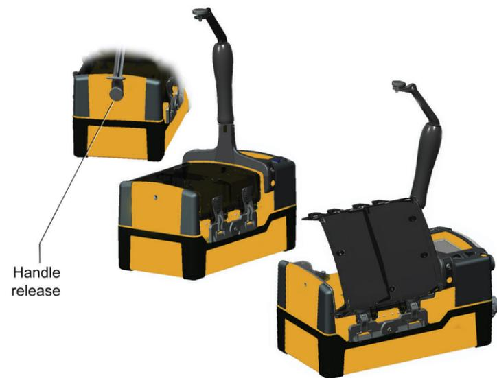
Figure 8: Opening the Chemcassette cartridge door
