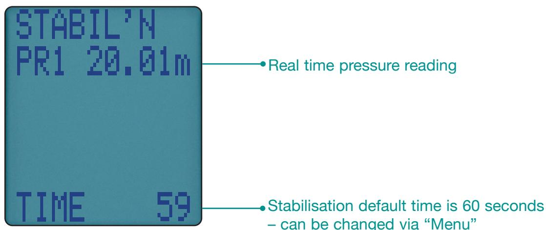
When complete press **←** to start the tightness test:
