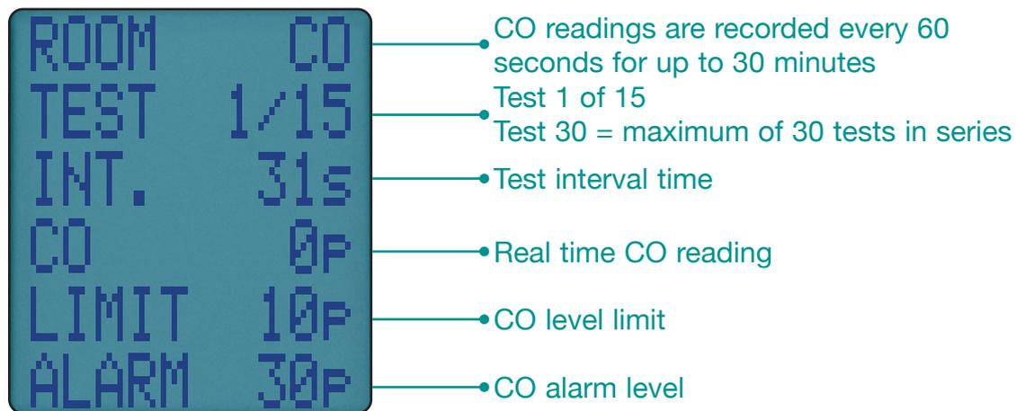
You can stop the Room CO test at any time by pressing **←**.
