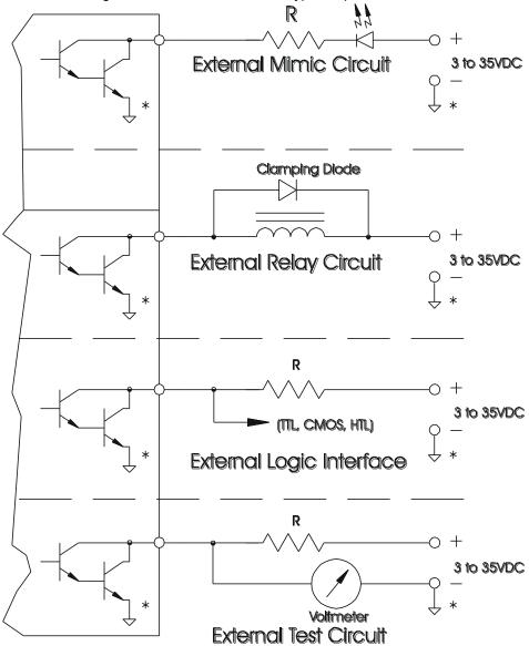
\* Note: All system commons (  $\stackrel{\bigcirc}{\downarrow}$  ) must be tied together.
