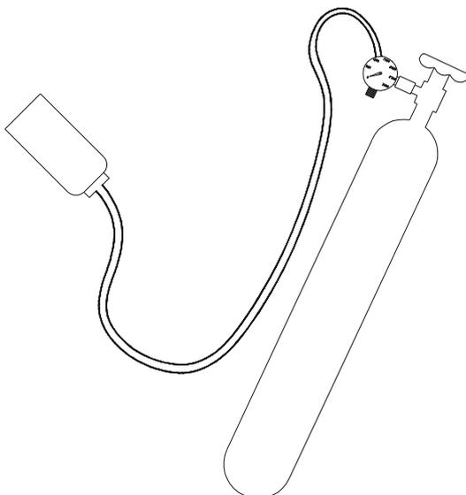
The General Monitors Portable Flow Calibrator is a compact, accurate and safe field calibrator which is used as an alternative to the H<sub>2</sub>S Field Calibrator for sensors located in high humidity environments. The calibrator uses gas bottles filled with known concentrations of H<sub>2</sub>S in dry air. Spare gas bottles are inexpensive and may be returned for refilling. Refer to the table below for the respective part numbers for ordering calibrators and replacement cylinders.
