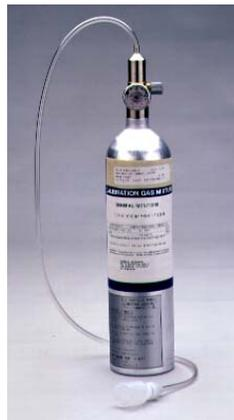
**Figure 21: Portable Purge Calibrator**
